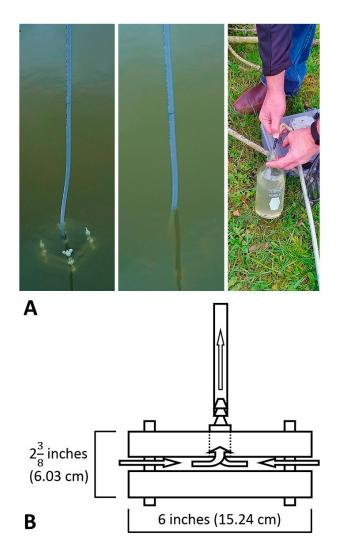
**Figure 3.** Use and action of the water sampler. (**A**) Lowering the sampler into the water by its tubing and subsequent sample collection in a rinsed and sterilized bottle. (**B**) Schematic diagram showing the mechanism of water sample collection (arrows indicate water flow). A major advantage of this design is that the water sample is pulled between the two acrylic squares within a space of 1 cm, allowing for high-resolution sampling and precise data collection.
