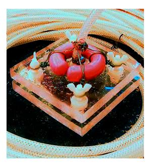
**Figure 4.** Water sampler fitted with additional ballast. The mass of the lead donut weight adds ballast to the sampler to ensure proper vertical orientation when lowered into the water column. Plastic coatings on the weight and wires prevent corrosion.
