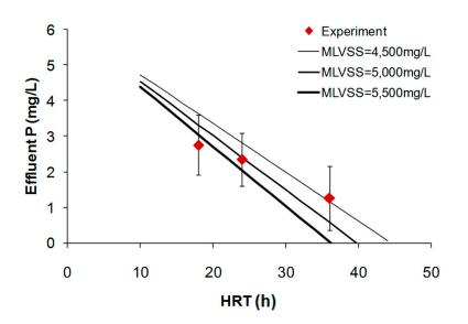
Figure 4. Effect of HRTs on effluent phosphate concentration.
