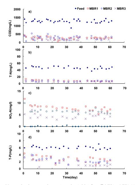
**Figure 2.** Water quality change over the experimental period ♦, influent □, MBR1 ○, MBR2: (a) COD; (b) T-N; (c) nitrate nitrogen; (d) T-P.
