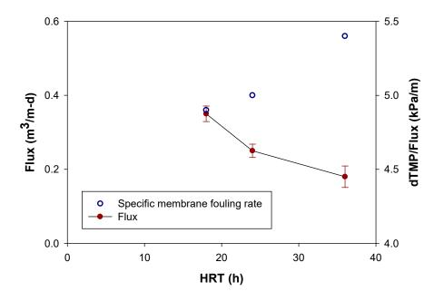
Figure 7. Effect of HRT on Membrane fouling rate and flux.
