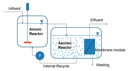
Figure 1. Schematic diagram of the MLE-type MBR.
