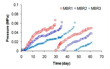
Figure 5. Transmembrane pressure profiles and cleaning.
