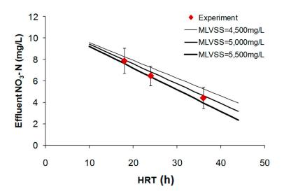
Figure 3. Effect of HRT on effluent nitrate nitrogen concentration.
