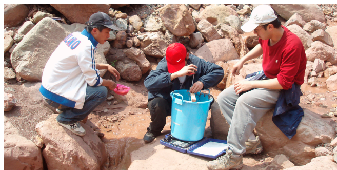
Figure 6. Obtaining the density in the field.
