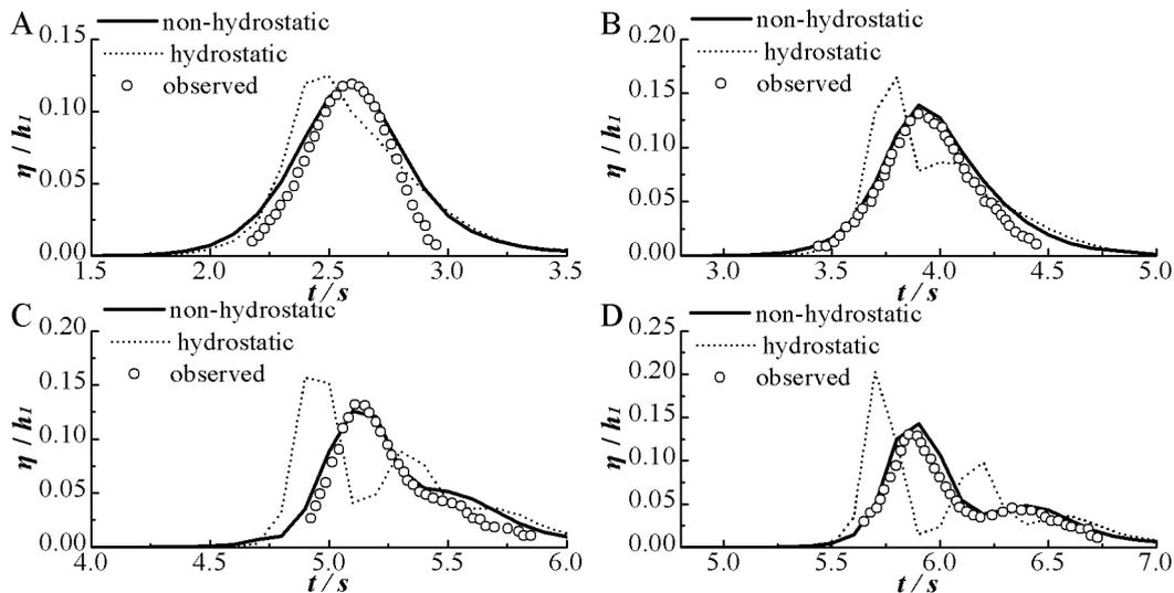
Figure 8. Simulated  $\eta/h_1$  by the non-hydrostatic (solid line) and hydrostatic model (dotted line); experimental data (circled) from Stations A, B, C, and D.
