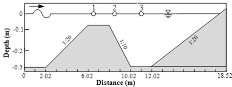
**Figure 11.** Sketch of the experimental setup of Nadaoka.
