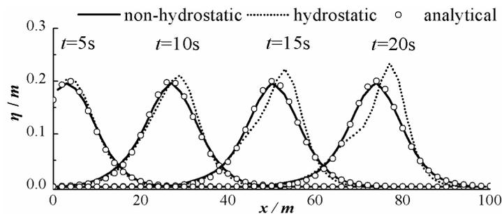
Figure 5. Simulated waveform by the non-hydrostatic (solid line) and hydrostatic model (dotted line); analytical waveform (circled) at different points in time ( $t = 5, 10, 15,$  and  $20$  s).
