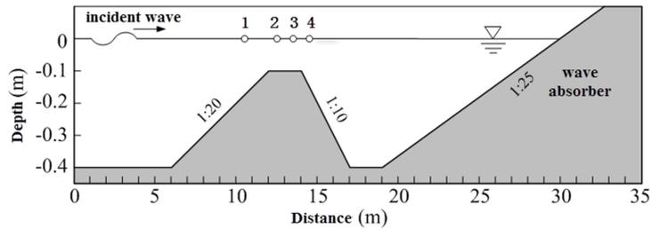
Figure 9. Sketch of the experimental setup of Beji.
