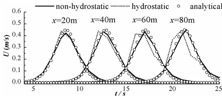
Figure 6. Simulated velocity  $U$  by the non-hydrostatic (solid line) and hydrostatic model (dotted line); experimental data (circled) at different locations ( $x = 20, 40, 60,$  and  $80$  m).
