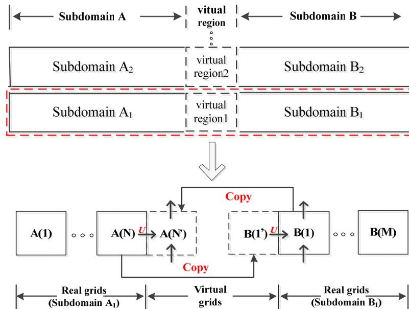
Figure 3. Domain decomposition and variable assignment of virtual grids.
