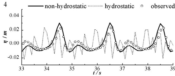
**Figure 10.** Simulated  $\eta$  by the non-hydrostatic (solid line) and hydrostatic model (dotted line); experimental data (circled) from Stations 1–4.
