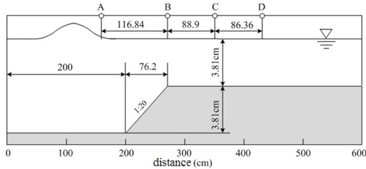
Figure 7. Sketch of the experiment setup of Madsen.
