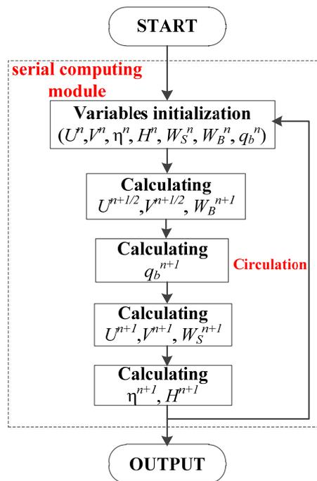
Figure 2. Solution steps of the non-hydrostatic model (serial computing).
