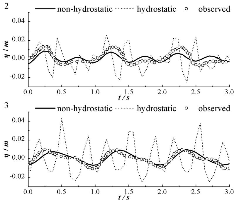
**Figure 12.** Simulated  $\eta$  by the non-hydrostatic (solid line) and hydrostatic model (dotted line); experimental data (circled) from Stations 1–3.
