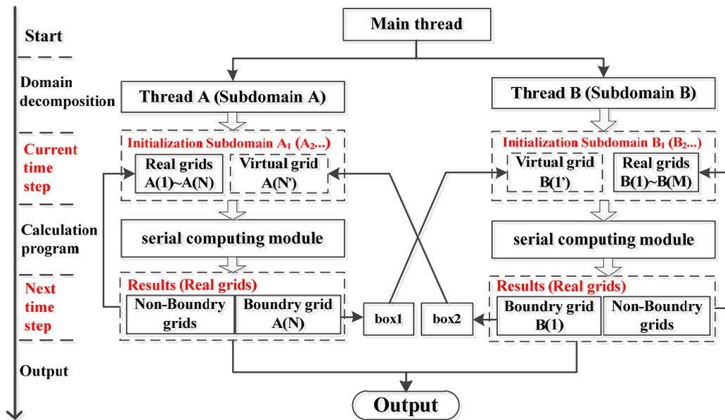
Figure 4. Solution steps of the non-hydrostatic model (parallel computing).
