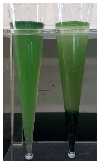
Figure 3. Clearing of algae suspension from the water column after 15 min of exposure to sonication and standing for 1 h. The left Imhoff cone is for the control and the right one for the treated suspension.
