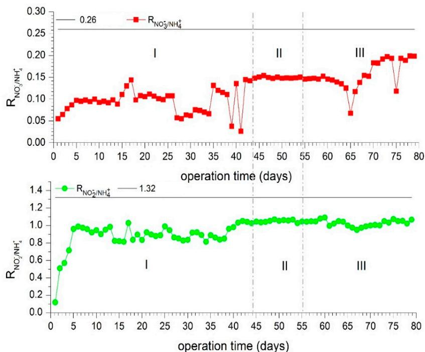
**Figure 3.** Ratios of nitrite consumption to ammonium consumption ( $R_{\text{NO}_3^-/\text{NH}_4^+}$ ) and nitrate production to ammonium consumption ( $R_{\text{NO}_2^-/\text{NH}_4^+}$ ) during the Anammox process.
