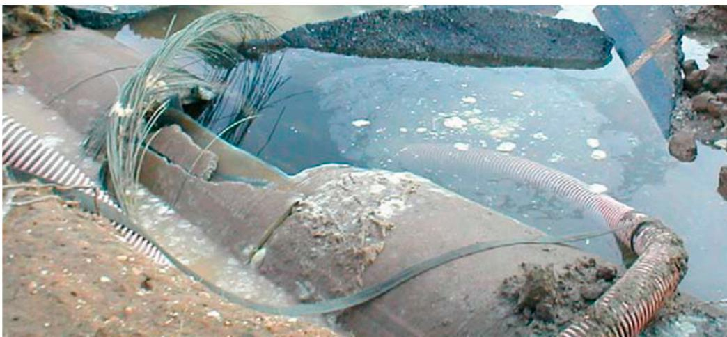
**Figure 1.** Rupture of the PCC pipe at chainage 0 + 465.80.
