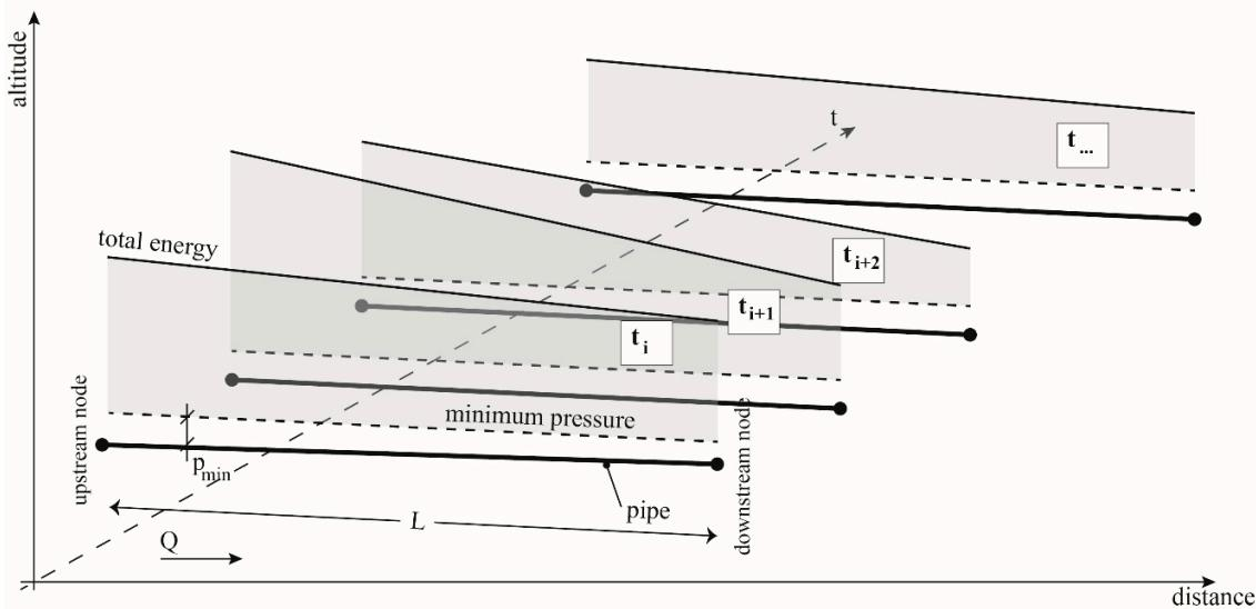
**Figure 1.** Energy excess at each point of a pipe, defined as the hydraulic head above minimum pressure, for several instances where a steady state is observed.
