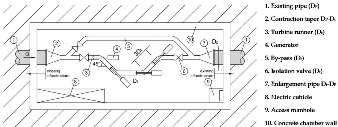
**Figure 7.** Sketch of the concrete chamber for the installation of a 5BTP (adapted from [18]). Up to four turbines can be installed with this design.
