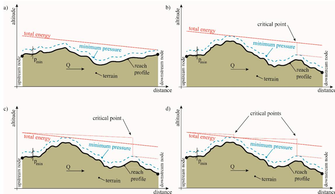
**Figure 2.** Examples of reaches. (a) Reach without available energy; (b) Reach with available energy; (c) Reach belonging to a closed network with available energy: effect of the extraction in one critical point; (d) Reach belonging to a closed network with available energy: effect of the extraction in two critical points.
