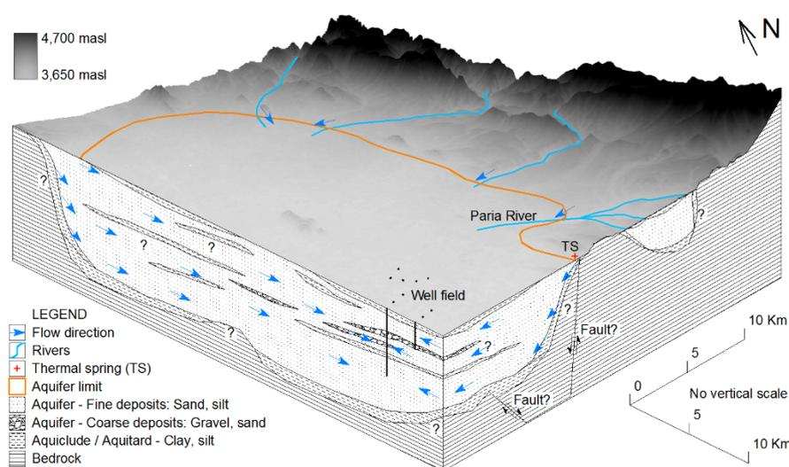
**Figure 2.** Schematic hydrogeological model of the Challapampa aquifer system (location in Figure 1b).
