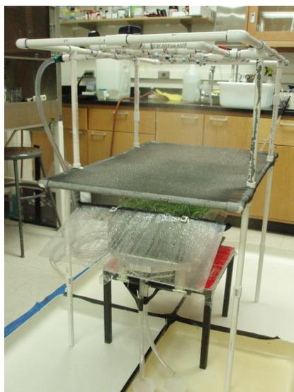
**Figure 1.** Complete laboratory-scale rainfall simulator and tilting soil bed system.
