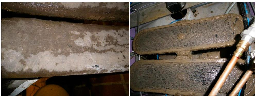
**Figure S2.** Pictures of aeration elements (left: calcified membrane tube; right: recurrently acidified membrane plate).
