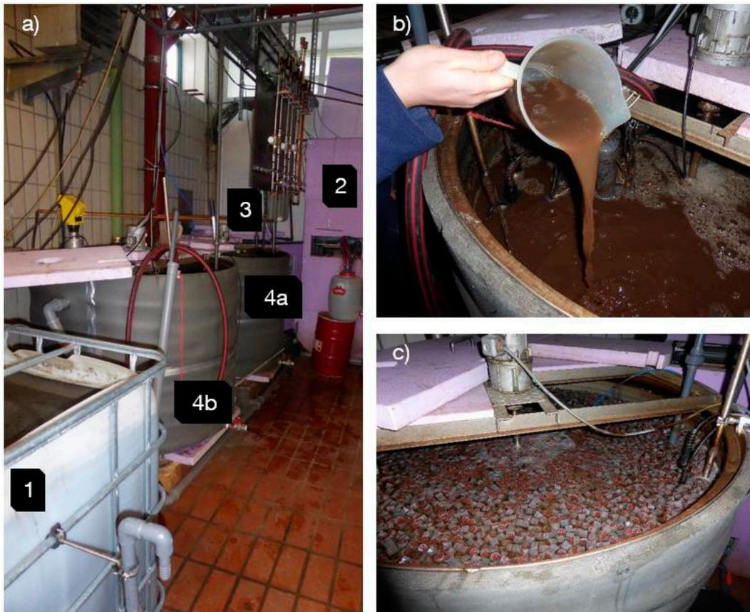
**Figure S1.** Two-stage deammonification pilot plant in Kempten (Allgäu): (a) Overview (1: Sedimentation; 2: Nitritation; 3: Buffer tank; 4a: Moving bed biofilm reactor (MBBR) with biofilm carriers; 4b: Sequencing batch reactor (SBR) with suspended sludge); (b) SBR with suspended sludge; (c) MBBR with biofilm carriers.
