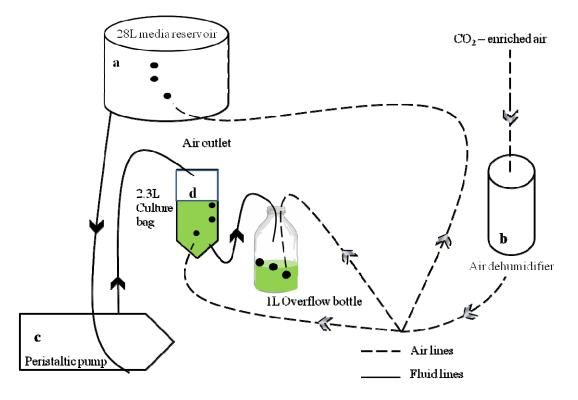
Teflon tubing was used for the overflow line as it is chemically inert, can be autoclaved and is very smooth, thereby avoiding settlement and/or adhesion of cells to the tube wall. The overflow silicone tubing was open to outside pressure by means of a 0.2  $\mu$ m air-filter on top. This ensured excess culture gently overflowed into the bottles rather than establishing a siphon.
