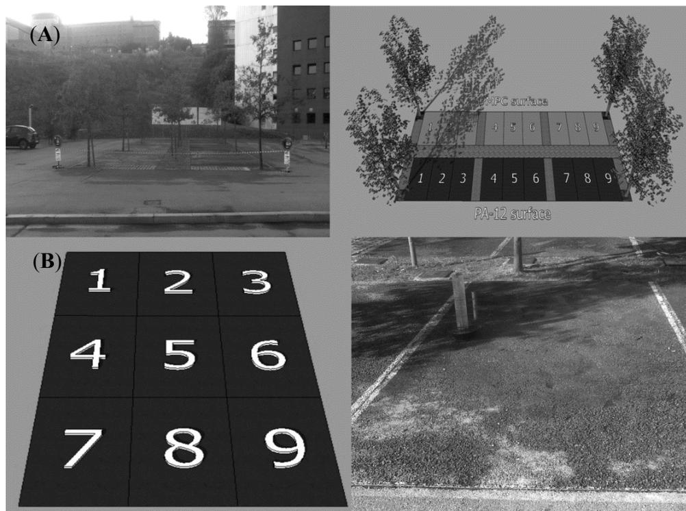
The infiltration capacity reduction was analyzed through the permeability results obtained now (after 5 years of operational life) in each test carried out using the LCS permeameter [18], comparing these values with those registered by [12] for the same porous surfaces when built (0.020 m/s for the case of the PMPC surfaces and 0.012 m/s for PA surfaces on average).
