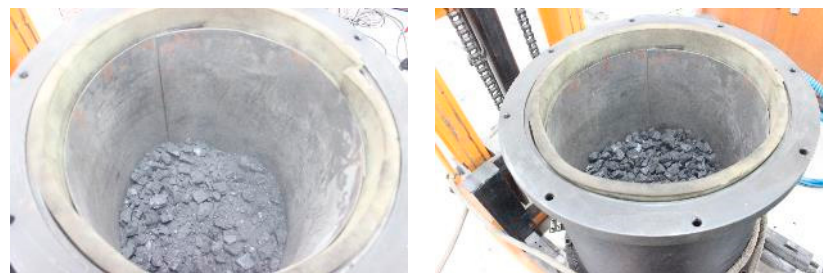
Figure 4. Microseismic compaction of broken-rock particles.
