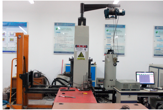
Figure 1. General view of the TAW-2000 kN Microcomputer-Controlled Electro-hydraulic Servo Triaxial Test System.
