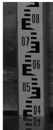
Figure 2. Grayscale image of the staff gauge after application of the weighted averaging method.
