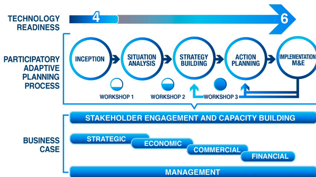
Figure 1. Participatory integrated planning of water reuse. Dark blue horizontal arrows indicate the sequential execution of the planning phases, while curved bottom arrows denote the iterative feedback loops from implementation monitoring and evaluation (M&E) back into strategy building and action planning. Partially filled circles represent stakeholder workshop progression, aligned with parallel Technology Readiness Level (TRL) advancement (top arrow), planning phases and business case steps (source; Authors' own).
