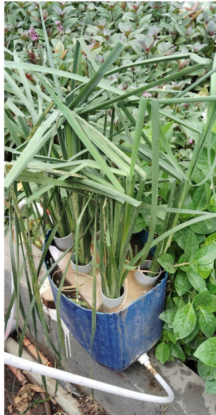
Figure 4. Typha angustifolia established in Container 1 (first stage) of the MTBRCW system, showing the bio-rack planting arrangement and the developed root matrix.
