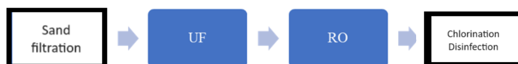
Figure 1. Scenario A reclaimed water treatment process. Source: Compiled by this research.
