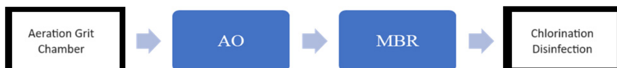
Figure 2. Scenario B reclaimed water treatment process. Source: Compiled by this study.
