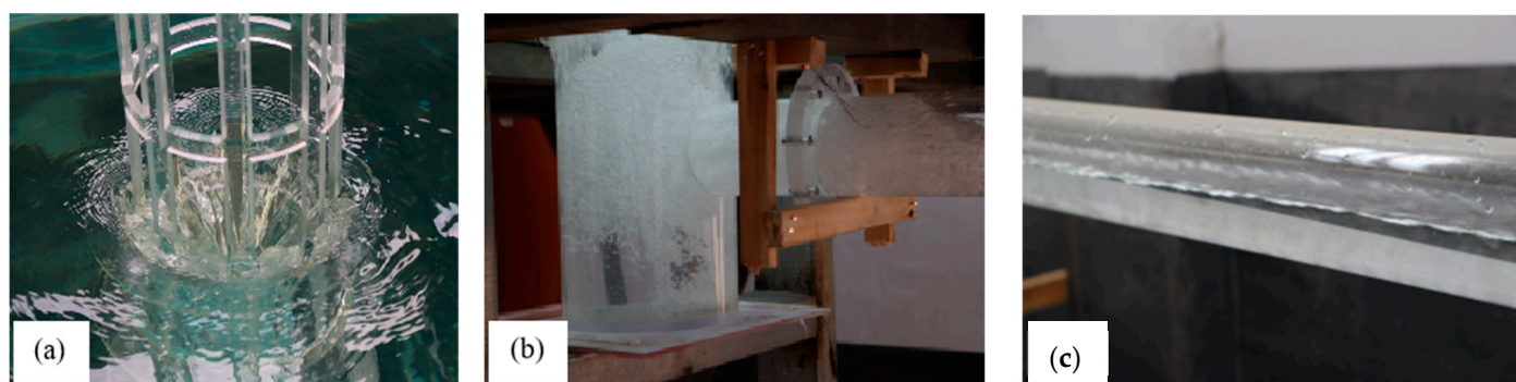
Figure 8. Flow regime at higher water head—partially pressurized flow; (a) shaft inlet flow pattern; (b) flow pattern of damper well; (c) flow pattern of flood drainage pipe.
