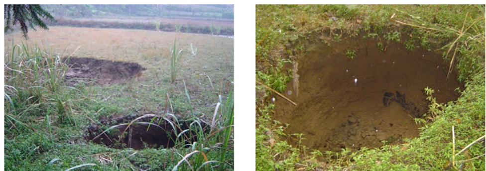
Figure 1. Field photographs showing typical karst collapse pits developed within thin overburden.
