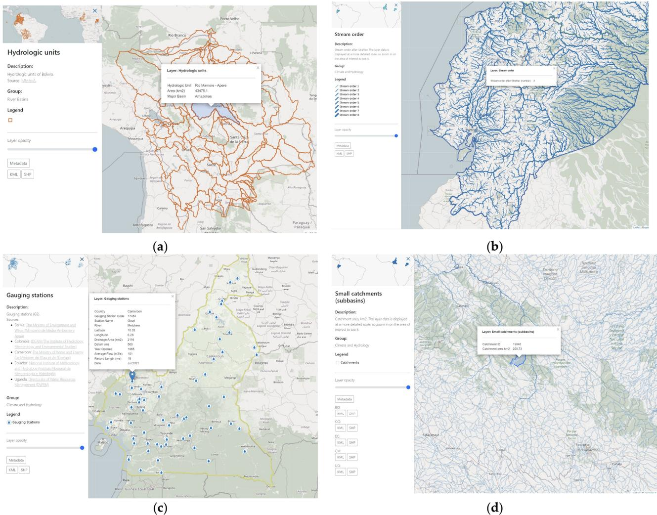
**Figure 5.** Hydrologic units (geospatial polygons) of Bolivia (a) and rivers and streams (geospatial polyline layer) with the Strahler stream order highlighted in Ecuador (b). River and stream gauging stations (GS) network in Cameroon (c). An extract of the small catchment area generated from the DEM in Bolivia (geospatial polygon layer). (d). A pop-up with a catchment area of 220.73 km<sup>2</sup> is highlighted.
