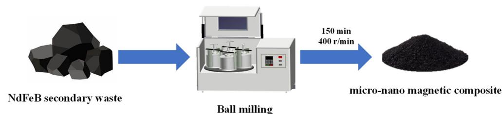
**Figure 1.** Process flowchart for preparing micro-nano magnetic composite materials.
