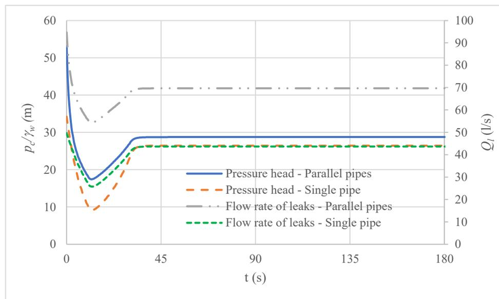
**Figure 6.** Comparison between single and parallel systems.
