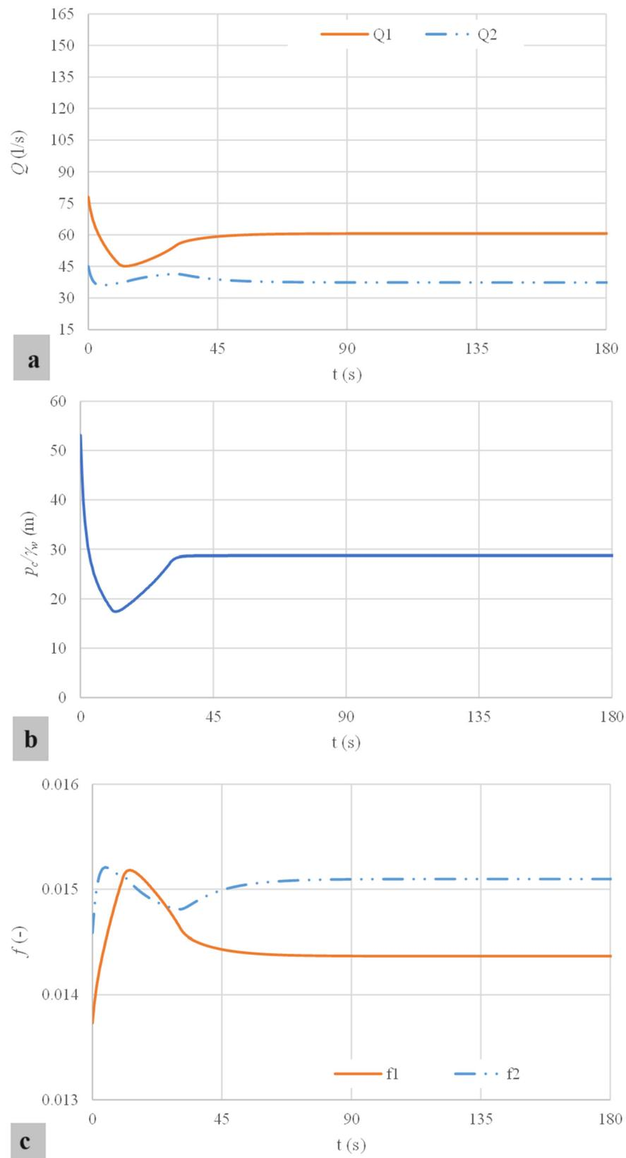
**Figure 4.** Results of main variables: (a) water flow rate; (b) pressure head; (c) friction factor.
