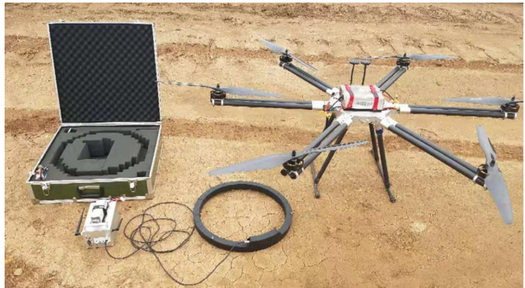
Figure 2. Ground-to-air electromagnetic signal receiving system based on rotary-wing UAV.
