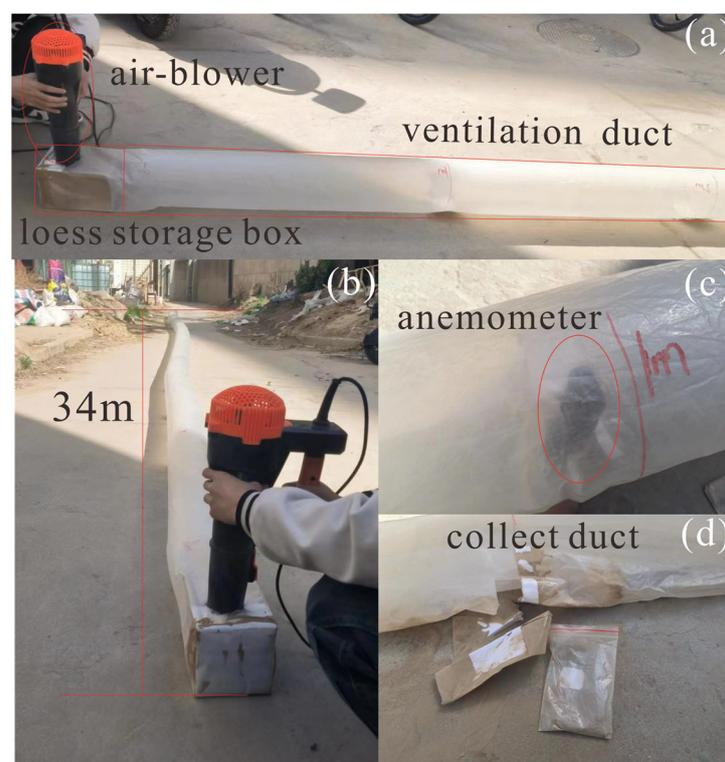
**Figure 2.** Experimental device and sampling: (a) components of the experimental device; (b) full view of the experimental device; (c) measurement of wind speed in the ventilation duct; (d) sampling after the experiment.
