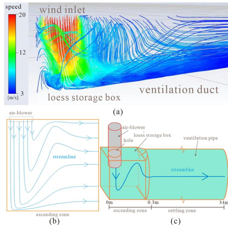
**Figure 3.** Flow field distribution inside the wind tunnel test device: (a) fluent output; (b) schematic of wind field redirection; (c) simplified representation of the wind field inside the experimental device.
