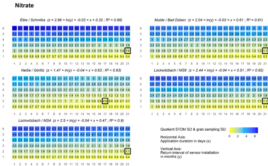
**Figure 9.** Quotient between the relative standard deviation of STOM and grab sampling for NO<sub>3</sub>-N; similar standard deviations between both sampling strategies are highlighted with black frames.
