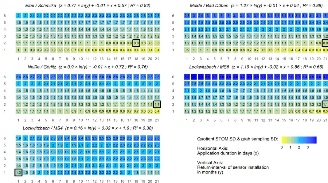
**Figure 11.** Quotient between the relative standard deviation of STOM and grab sampling for dissolved oxygen; similar standard deviations between both sampling strategies are highlighted with black frames.
