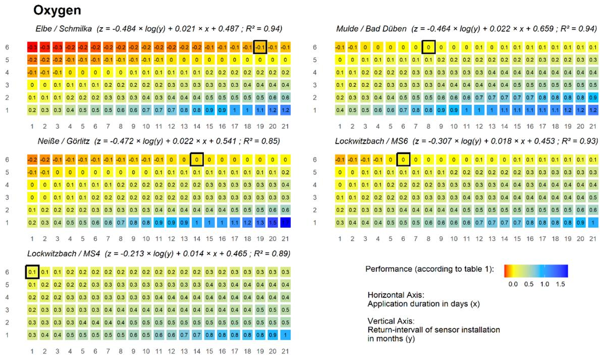
**Figure 6.** Comparison of STOM and grab sampling for dissolved oxygen. Values were calculated according to Figure 3; break even points from regression model are highlighted with black frames.
