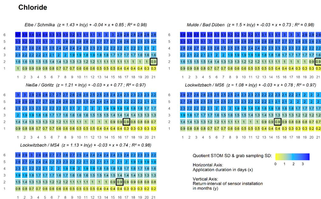
**Figure 10.** Quotient between the relative standard deviation of STOM and grab sampling for chloride; similar standard deviations between both sampling strategies are highlighted with black frames.
