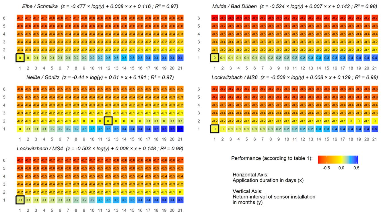
**Figure 4.** Comparison of STOM and grab sampling for nitrogen-nitrate. Values were calculated according to Figure 3; break even points from the regression model are highlighted with black frames.
