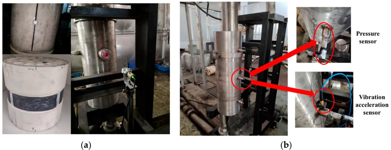
**Figure 30.** Sensors for rotary speed, pressure and vibration acceleration. (a) Rotary speed sensor; (b) pressure and vibration sensor.
