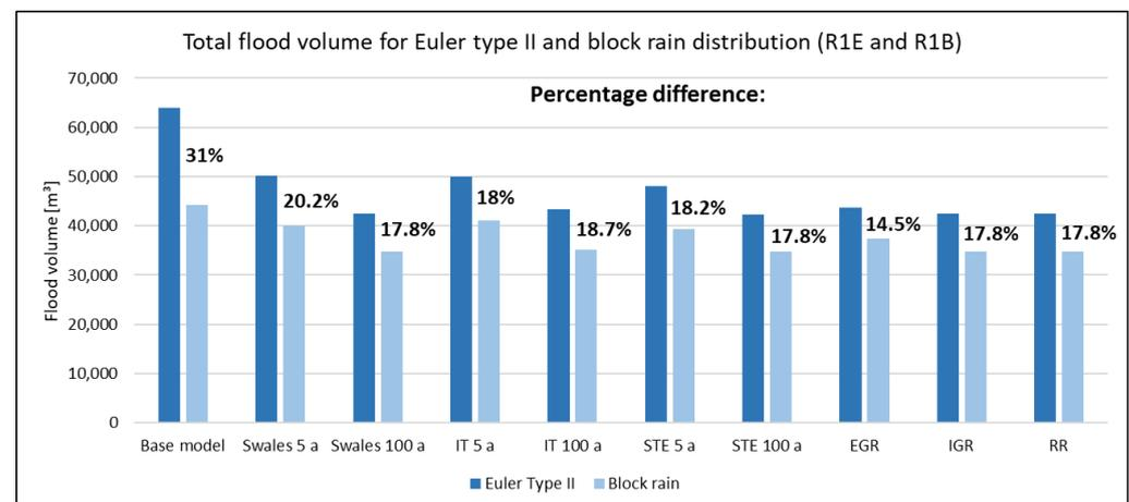
**Figure 9.** Comparison of the total flood volume for the base model and various NBSs (implementation degree: 100%) between the Euler type 2 and block rain distribution for R1E and R1B, respectively.
