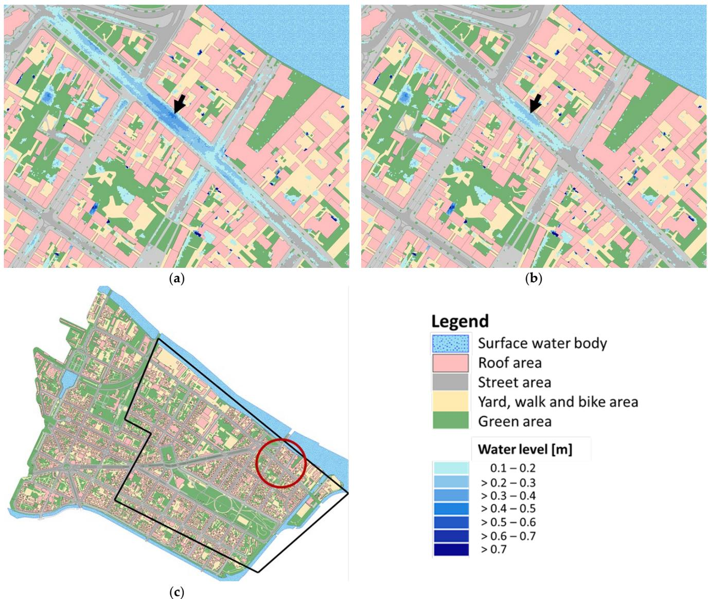
**Figure 11.** Maximum flood heights in the center of flooding with R1E, and the black arrows indicate the lowest point in the street area: (a) homogenous distribution of retention roofs, implementation degree: 50.3%; (b) heterogenous distribution of retention roofs, implementation degree: 50.3%; and (c) center of flooding marked by a red circle. In the black polygon, 50.3% of the roofs are located.
