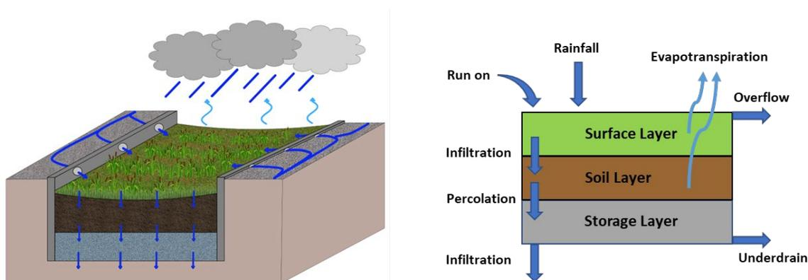
**Figure 3.** Layer structure of the SUDS element bio-retention cell in InfoWorks ICM/SWMM (own illustration based on Rossman and Huber [36]).
