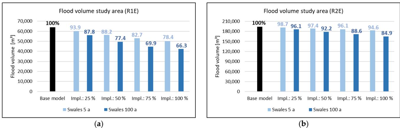
**Figure 7.** Total flood volume in the study area for the base model and with swales (dimensioned to T = 5 and 100 a) with different degrees of implementation: (a) total flood volume for R1E (precipitation height: 48.9 mm) and (b) total flood volume for R2E (precipitation height: 100 mm).
