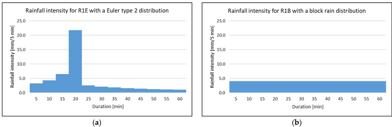
**Figure 6.** (a) Euler type 2 rainfall distribution; (b) block rain distribution.
