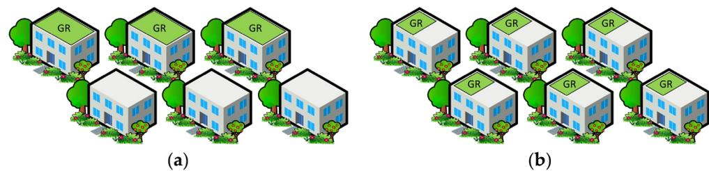
**Figure 5.** (a) Heterogeneous distribution of the green roofs: 50% of the roof areas implemented as green roofs; (b) homogeneous distribution: 50% of each individual roof area is designed as a green roof.
