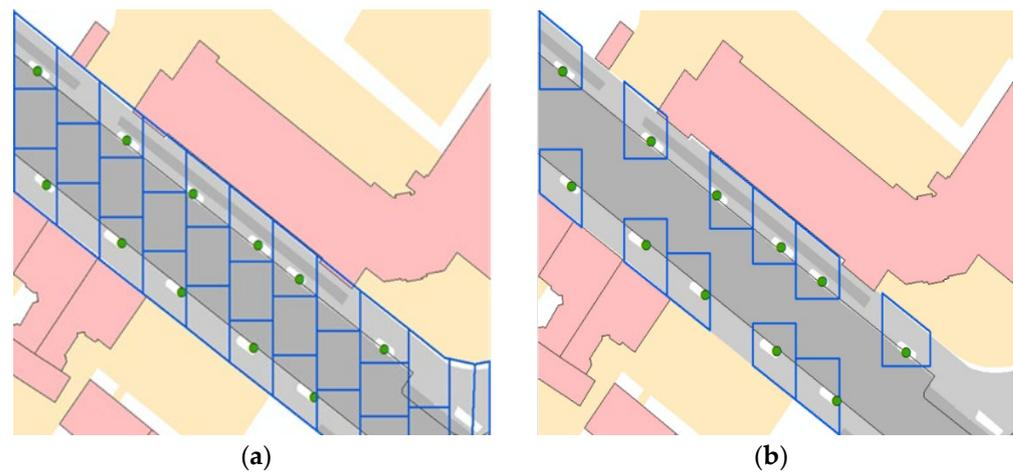
**Figure 4.** (a) Street area divided into 120 m<sup>2</sup> polygons (blue) and the locations of street trees (green); (b) selected polygons that represent subcatchments connected to a tree trench in the model.
