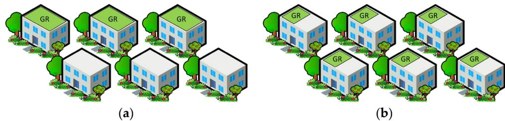
**Figure 5.** (a) Heterogeneous distribution of the green roofs: 50% of the roof areas implemented as green roofs; (b) homogeneous distribution: 50% of each individual roof area is designed as a green roof.
