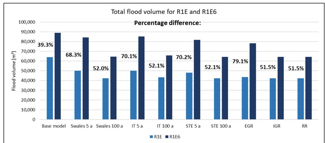
**Figure 10.** Comparison of the total flood volume for the base model and various NBSs (implementation degree: 100%) between R1E and R1E6.
