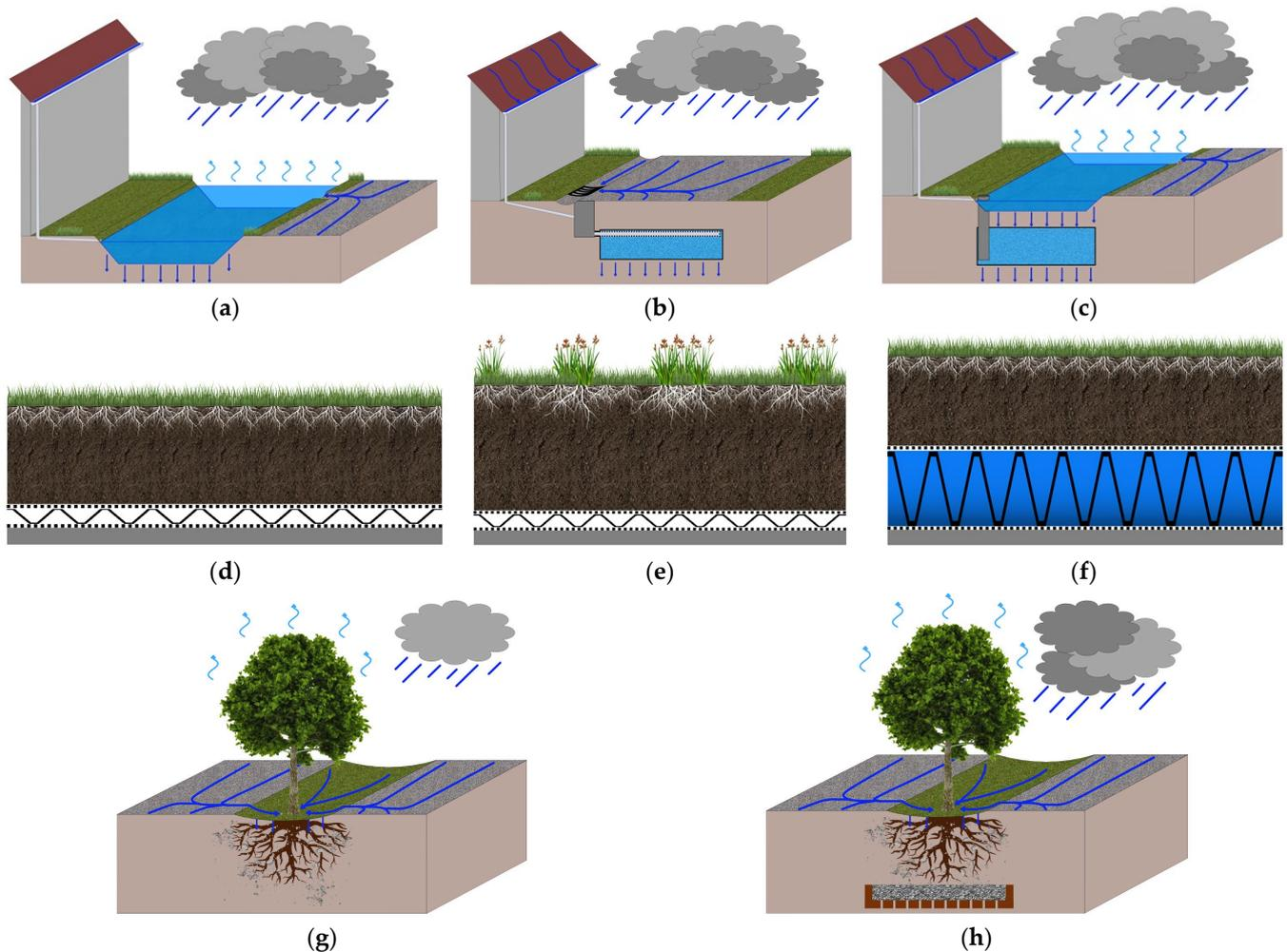
**Figure 2.** Investigated decentral NBSs. Infiltration systems: (a) swale; (b) infiltration trench; (c) swale–trench–element; green roofs: (d) extensive green roof; (e) intensive green roof; (f) retention roof; tree locations: (g) tree pit; and (h) tree trench.
