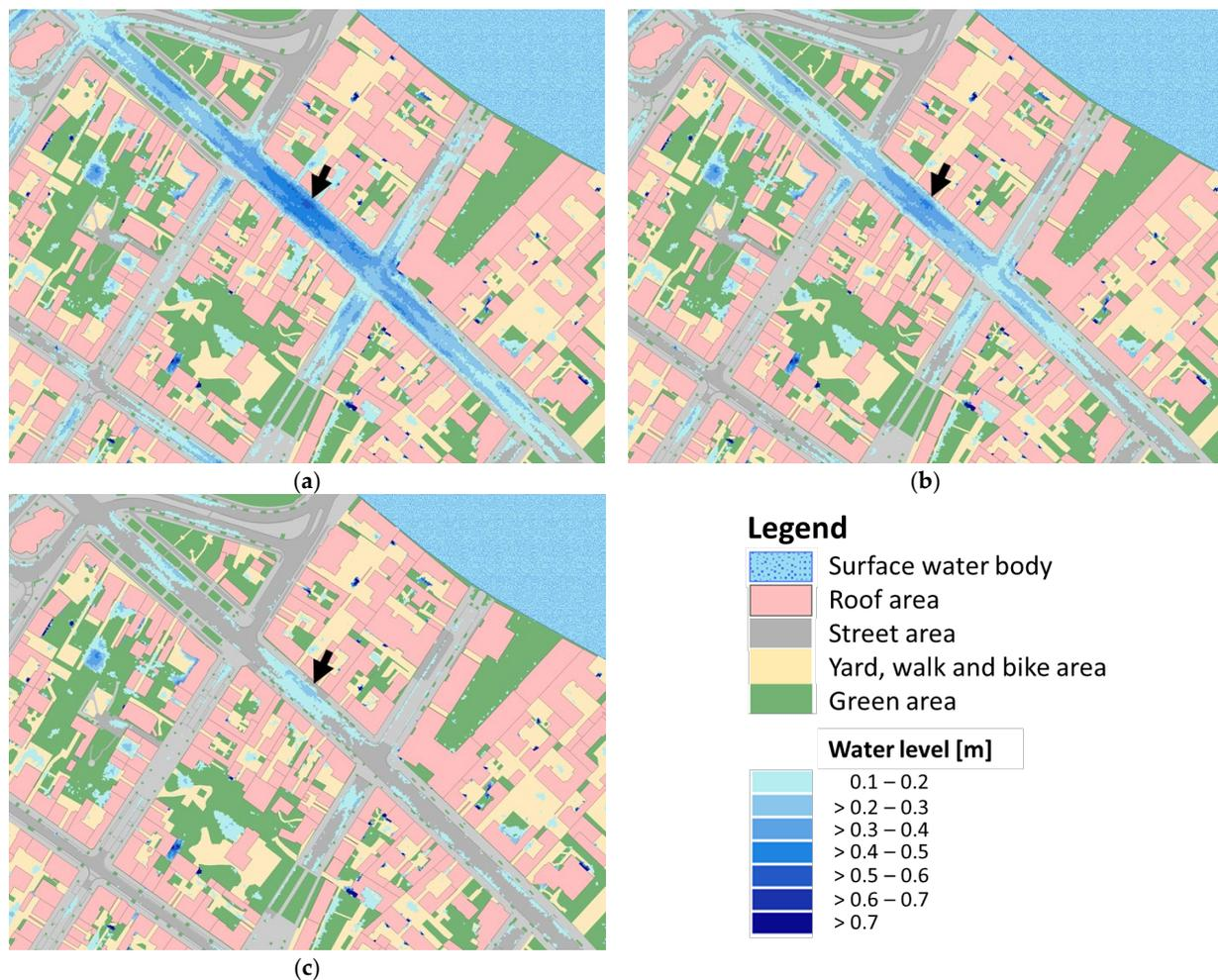
**Figure 8.** Maximum flood heights in the center of flooding: (a) base model; (b) swales ( $T = 100$  a), degree of implementation: 50%; and (c) swales ( $T = 100$  a), degree of implementation: 100%. The black arrows indicate the lowest point in the street.
