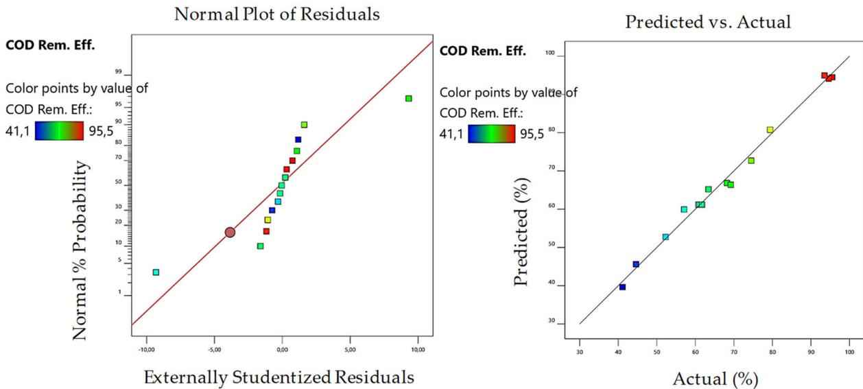
**Figure 2.** Normal probability residual plot and predicted vs. actual plot based on chemical oxygen demand (COD) removal efficiency values for the UV/Fenton process.
