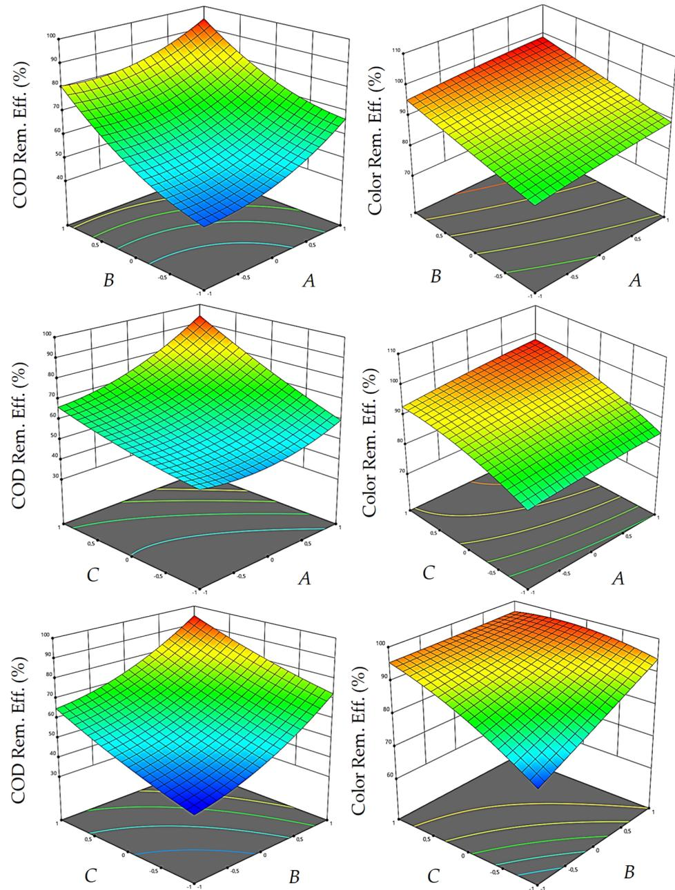
A: Time (min), B: UV Power (W), C:  $\text{H}_2\text{O}_2/\text{Fe}^{2+}$  ratio
