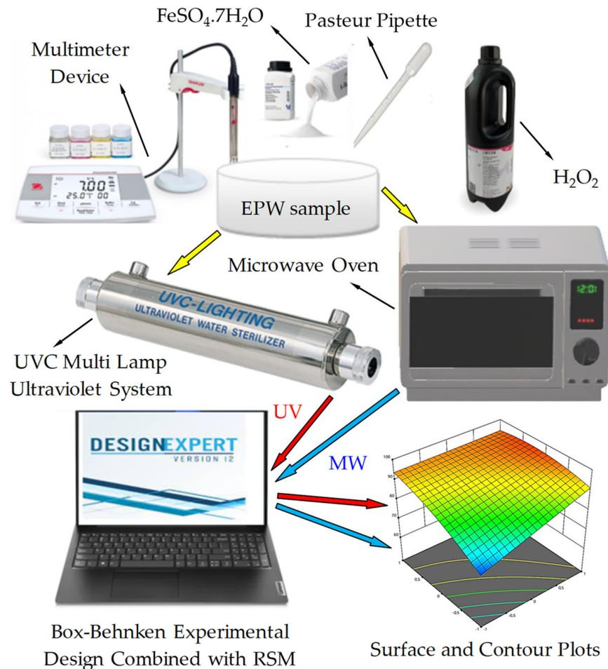
**Figure 1.** Pictorial diagram of the treatment process used for the advanced oxidation of EPW.
