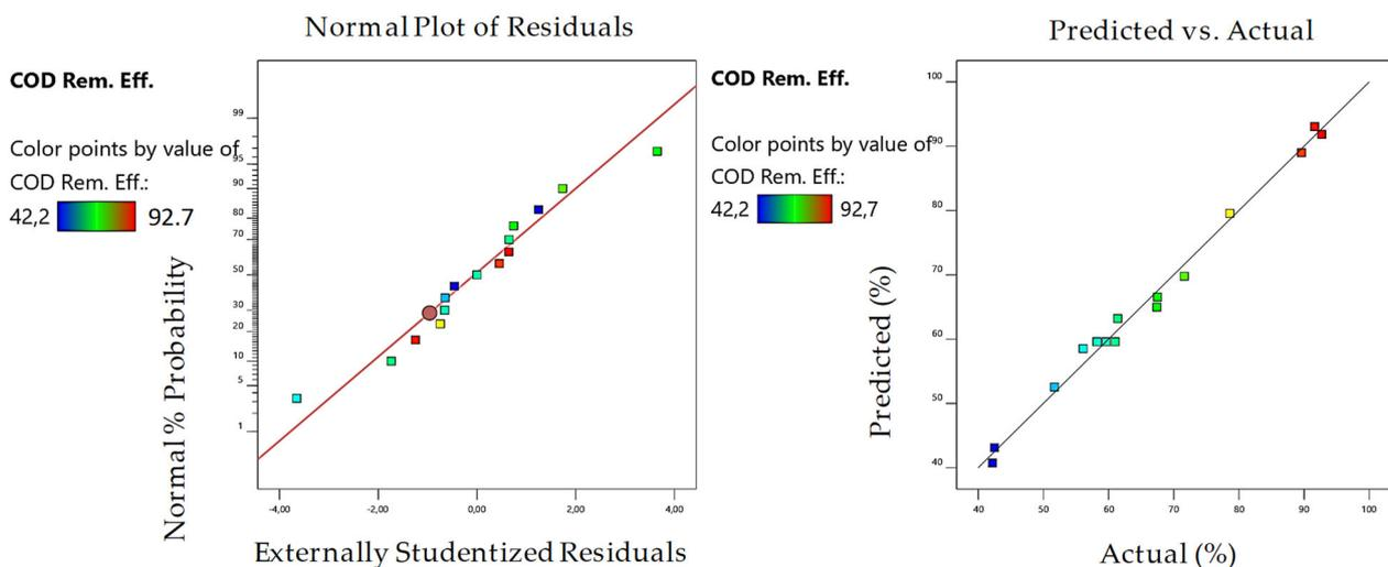
**Figure 5.** Normal probability residual plot and predicted vs. actual plot based on chemical oxygen demand (COD) removal efficiency values for the MV/Fenton process.
