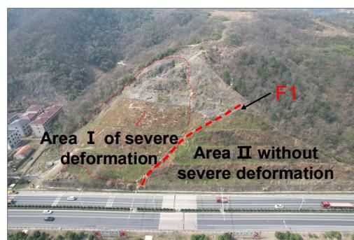
**Figure 6.** Landslide deformation area.
