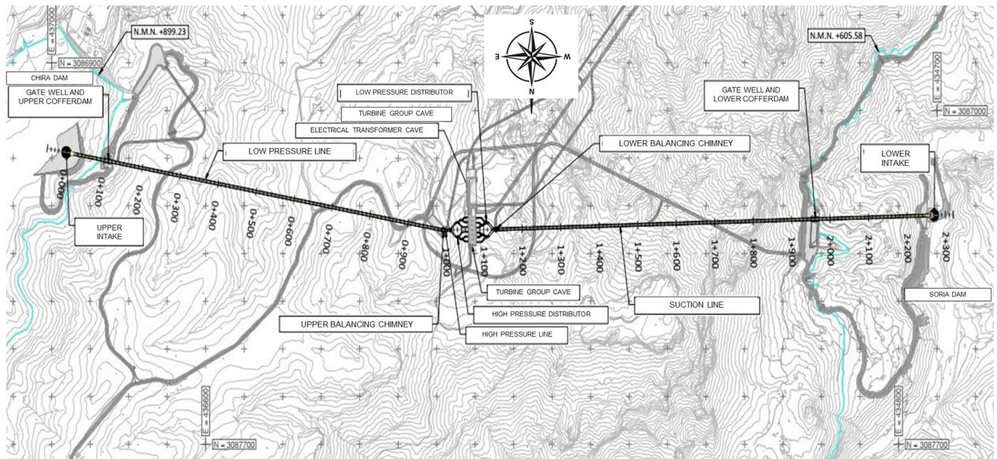
**Figure 5.** General plan of the Hydraulic Circuit, with the Chira reservoir on the right and the Soria reservoir on the left in this image (image oriented south instead of north).
