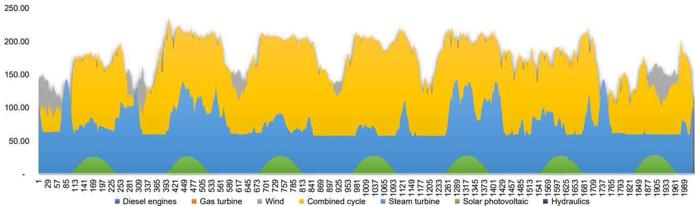
**Figure 8.** Instantaneous production (MW) from 16 to 22 August 2021 [18].
