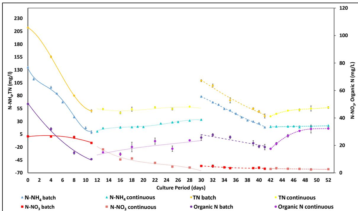
Figure 11. Time profiles of various nitrogen form concentrations during the continuous operation of the ATPBR.
