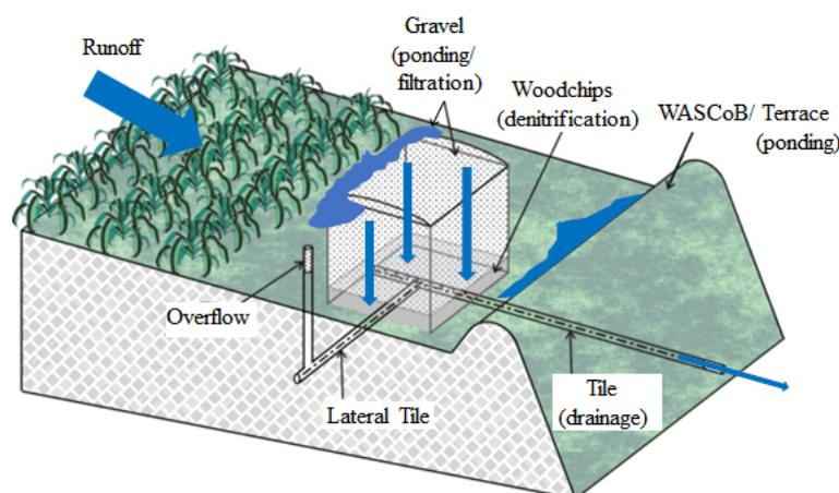
**Figure 1.** An alternative tile intake consisting of a buried column of gravel over a layer of woodchips. Blue arrows represent flowpaths of water. The blue, irregular shapes represent ponding of water.
