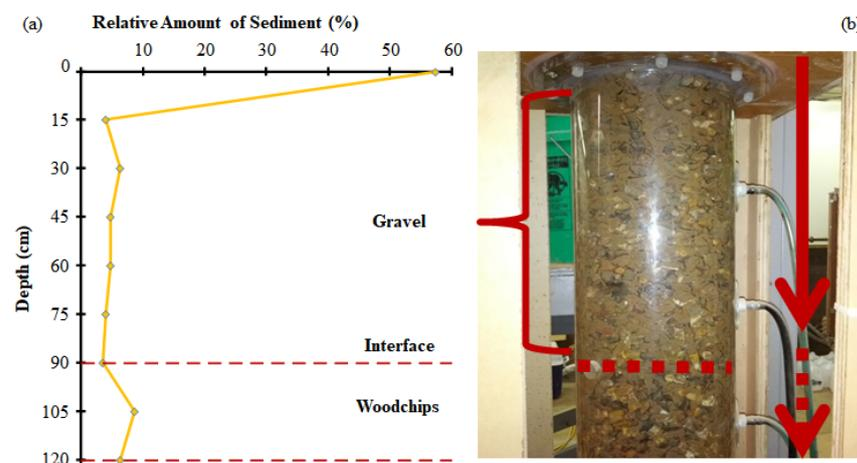
**Figure 7.** (a) Mass of deposited sediment in the permeameter after all runs. (b) Visible intrusion of sediment following a sediment test. Arrows indicate direction of flow.
