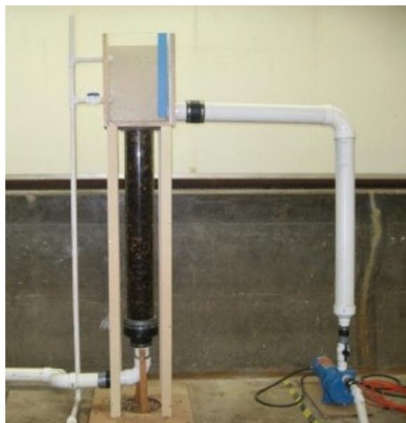
**Figure 5.** Physical model of an ATI. This permeameter was developed to determine the effective hydraulic conductivity of the ATI and quantify its filtering efficiency through the pea gravel and woodchips.
