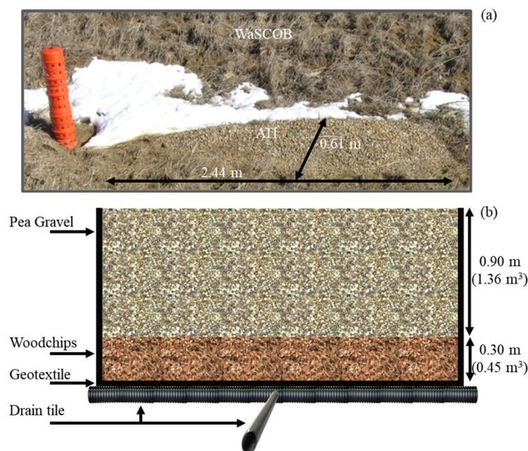
**Figure 3.** (a) An installed ATI at the Iowa County site. At the surface, only the pea gravel is visible. The orange pipe was left as a safety precaution. The holes on the lower half were blocked. (b) A vertical cross section of the ATI with 0.90 m of gravel over 0.30 m of woodchips.
