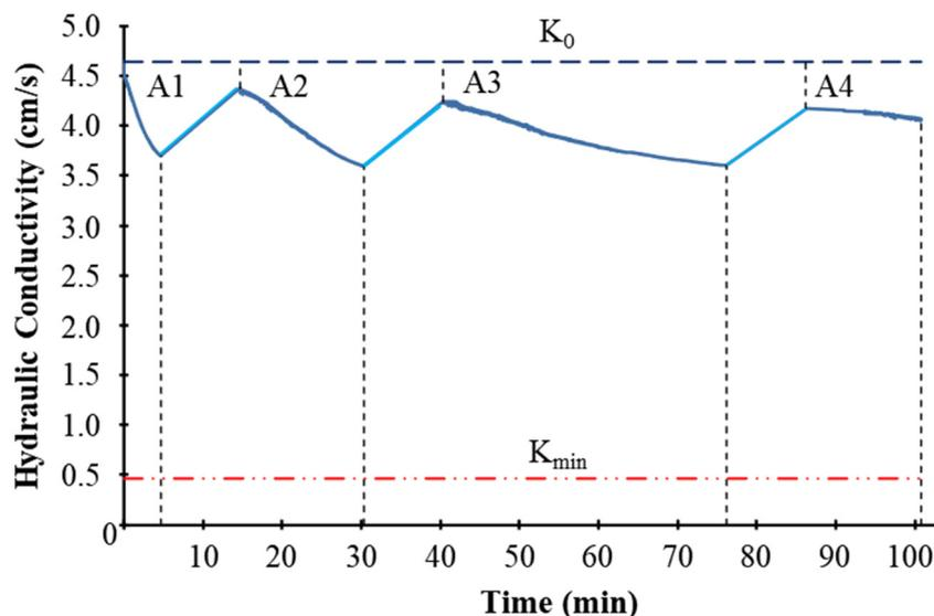
**Figure 9.** Time series of hydraulic conductivity,  $K$ , over consecutive runs. The initial hydraulic conductivity of the gravel–woodchip matrix,  $K_0$ , averaged  $4.59 \text{ cm/s} \pm 0.36 \text{ cm/s}$ . The minimum hydraulic conductivity value ( $K_{\min}$ ) is considered the minimum value at which water passes through the matrix. The value for  $K_{\min}$  of  $0.10 \times K_0$  was adopted from [2,33].
