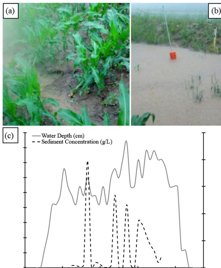
**Figure 10.** Sampled runoff event. (a) A rill that formed delivered water to the ATI. (b) Ponding near the control intake. (c) Water depth measured with the pressure transducer in the drain tile below the ATI. The maximum depth of 4.5 cm corresponds to 35.4% of the pipe cross-sectional area.
