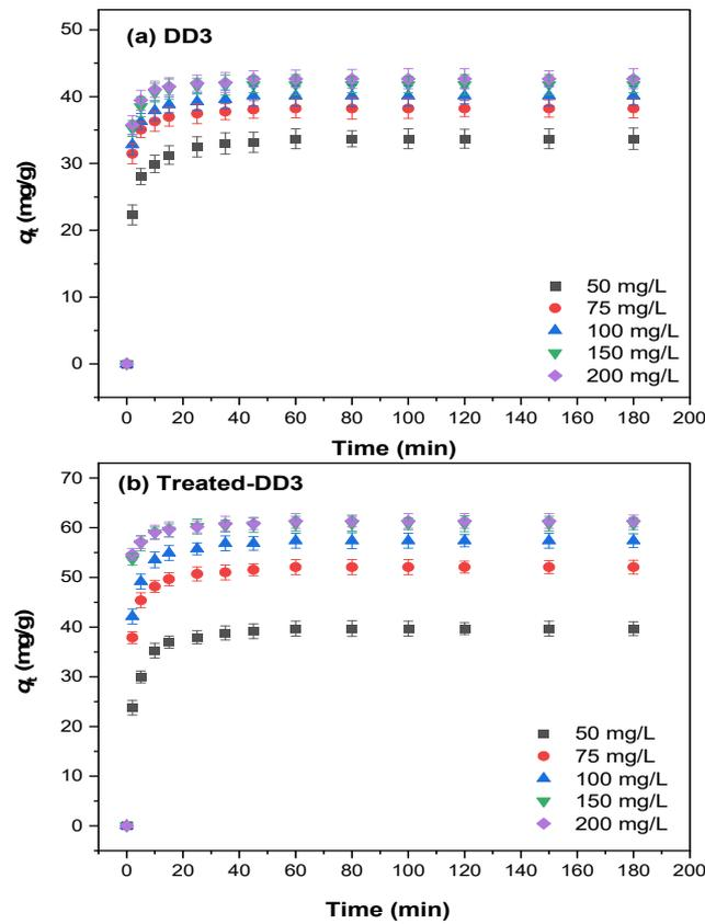
**Figure 6.** Effect of contact time and initial concentration of MB on the adsorption capacity of (a) DD3 and (b) treated-DD3 ( $m/V = 1 \text{ g/L}$ ,  $25 \pm 3 \text{ }^\circ\text{C}$ , and unadjusted pH).
