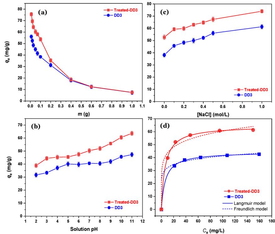
**Figure 5.** (a–c) Effect of adsorbent doses (solid/liquid ratios), solution pH, and ionic strength on the adsorption of MB onto DD3 and treated-DD3; and (d) dye adsorption isotherm by DD3 and treated-DD3.
