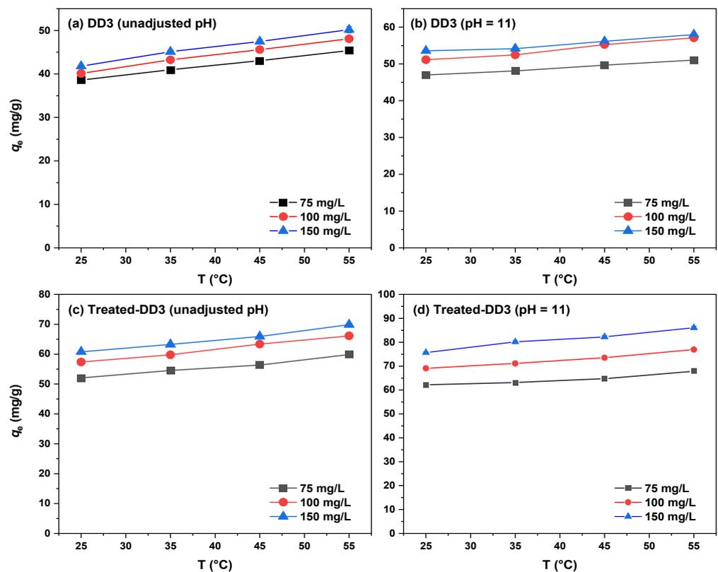
Figure 7. Effect of temperature on the adsorption capacity of the MB dye onto (a,b) DD3 and (c,d) treated-DD3 at different solutions' pH and initial dye concentrations.
