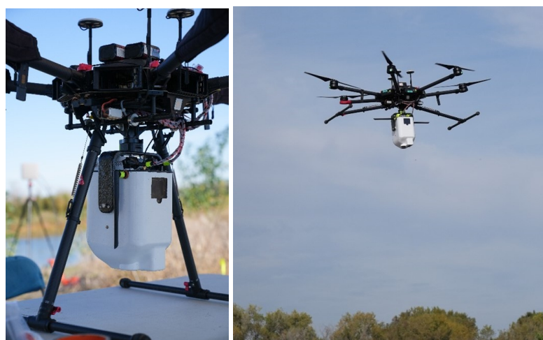
Figure 3. Images of the DJI Matrice 600 Pro hexacopter equipped with the River Observing System (RiOS) payload. Photographs by Massimo Vespignani, NASA, used with permission.
