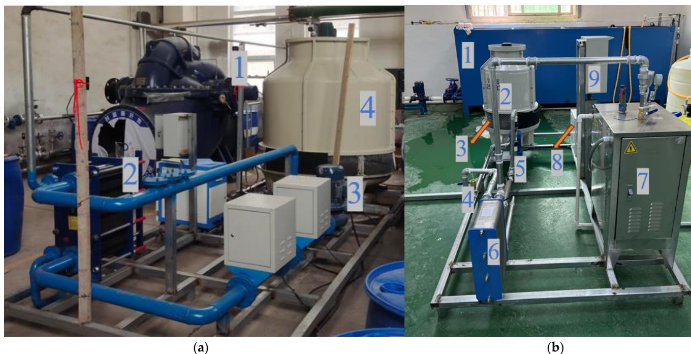
Figure 3. (a) Industrial circulating water cooling water system 1 Water supply pipe; 2 Heat exchanger; 3 Circulating water pump; 4 Cooling tower (b) Physical diagram of a small-scale industrial circulating water composite descaling experimental platform 1 Water storage and replenishment tank; 2 Cooling tower; 3 Scaling machine; 4 Valve; 5 Electrical machinery; 6 Heat exchanger; 7 Temperature control device; 8 Electromagnetic device; 9 Power control cabinet.
