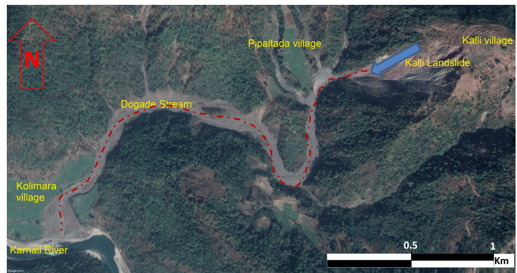
Figure 5. Kalli landslide, occurring at Kalli village, and the debris runout along the Dogade stream to the Karnali river. The blue arrow indicates the landslide mobilized from the crown area at Kalli village. The red line indicates potential debris flow path along the Dogade stream. The upstream portion of the Dogade stream from the Kalli landslide area cannot be noticed clearly as the channel is constricted; but the portion between the Kalli landslide and the Karnali river is evident due to the widened channel resulting from the debris flow. A very wide debris fan along with the Karnali river constriction at the confluence point of the Dogade stream and the Karnali river due to debris deposit can be clearly observed.
