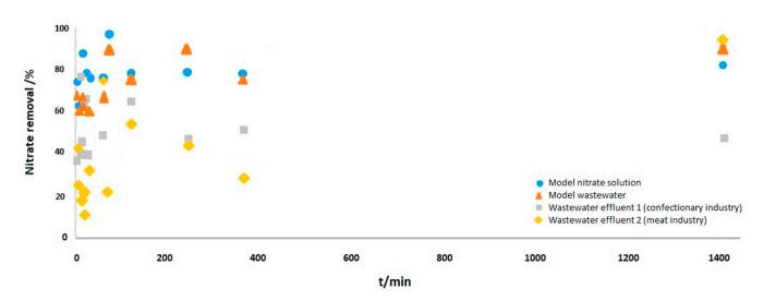
Figure 5. Effects of contact time on nitrate removal by MS.
