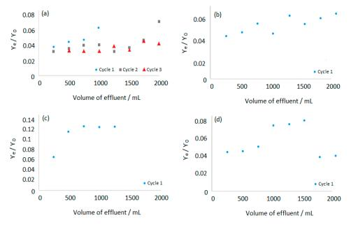
**Figure 6.** Breakthrough curves for the adsorption of nitrate ions from (a) model nitrate solution, (b) model wastewater, (c) real wastewater from the confectionery industry, and (d) real wastewater from the meat industry on MSS.
