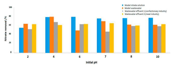
**Figure 4.** Effects of pH on nitrate removal by MSS ( $Y_{nitrate} = 30 \text{ mg L}^{-1}$ ,  $\gamma_{adsorbent} = 4 \text{ g L}^{-1}$ ,  $T = 25 \,^{\circ}\text{C}$ ,  $V_{nitrate solution} = 50 \text{ mL}$ , t = 120 min).
