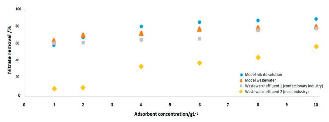
**Figure 2.** Effects of MSS concentration on nitrate removal ( $Y_{nitrate} = 30 \text{ mg L}^{-1}$ ,  $T = 25 \, ^{\circ}\text{C}$ ,  $V_{nitrate solution} = 50 \, \text{mL}$ ,  $t = 120 \, \text{min}$ ).
