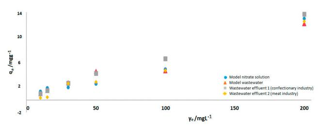
**Figure 3.** Effects of initial N-NO<sub>3</sub> concentration on nitrate removal by MSS ( $\gamma_{adorbent} = 4 \text{ g L}^{-1}$ , T = 25 °C,  $V_{nitrate solution} = 50 \text{ mL}$ , t = 120 min).
