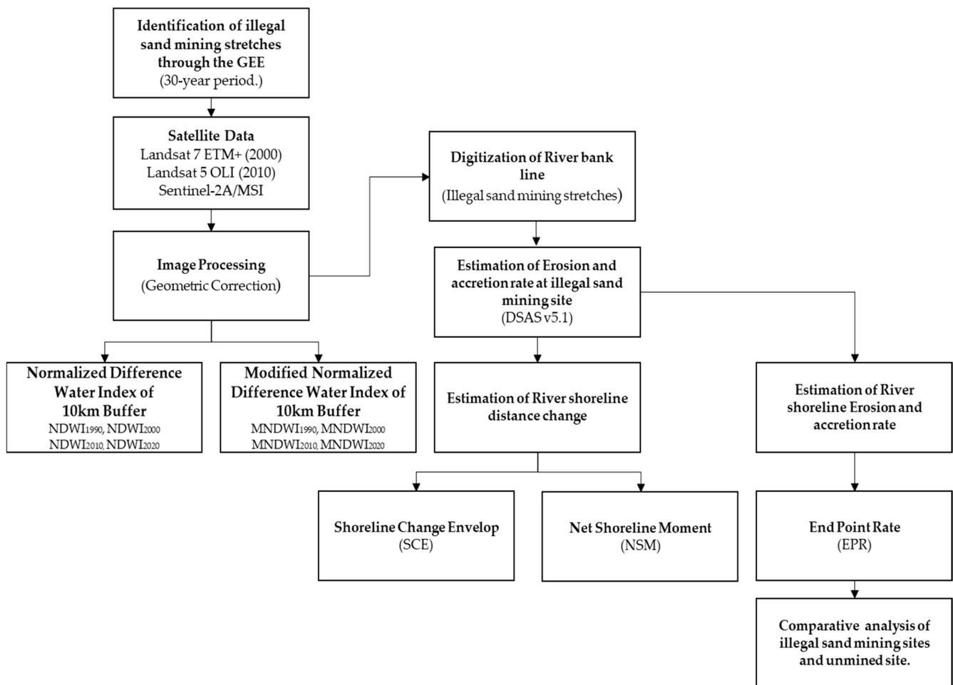
**Figure 4.** Flowchart diagram illustrating the methodology for evaluating erosion and accretion at mining sites. The diagram outlines the steps to analyze the satellite images and geospatial data, including spectral indices and a digital shoreline analysis system (DSAS) to calculate shoreline erosion and accretion rates.
