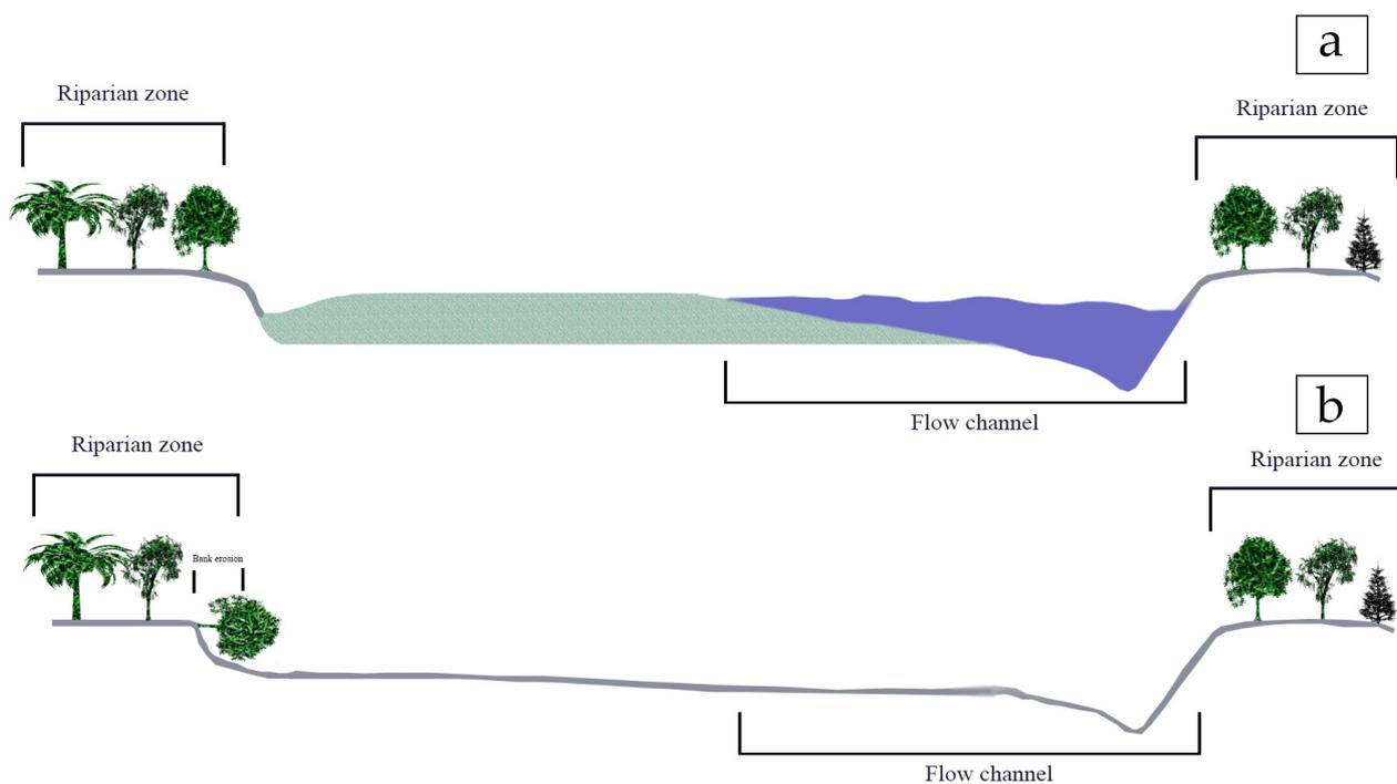
**Figure 2.** Comparison of channel cross-sections. (a) shows a typical sand–gravel bar inside the low-flow channel, while (b) depicts the impact of uncontrolled mining resulting in a large shallow channel with severe bank erosion.
