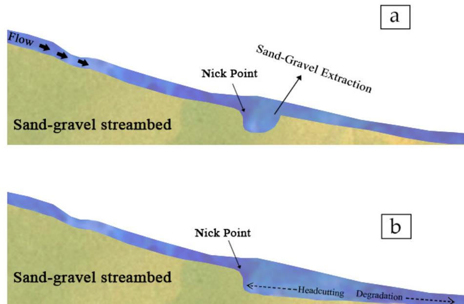
**Figure 1.** Illustration of a sand and gravel streambed and the impact of illegal sand mining. (a) Nick points, where the streambed is abruptly lowered due to pit excavation, can be seen. (b) Downstream from the nick point, the streambed deteriorates when flow rates are high due to the lack of sediment replenishment caused by the mining.
