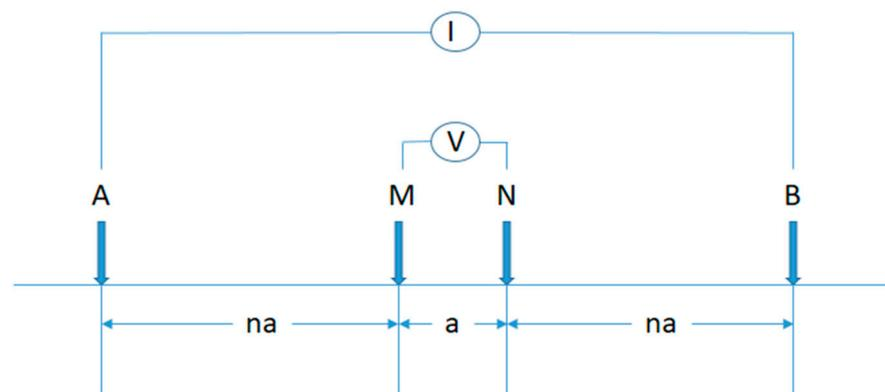
**Figure 6.** Electrode arrangement for the Schlumberger configuration. AB represent the current electrode pairs and MN represent the potential electrode pairs; I is the current source and V is the volt meter; a represents the space between the moving MN electrodes and na represents the moving space in between the AB current electrodes.
