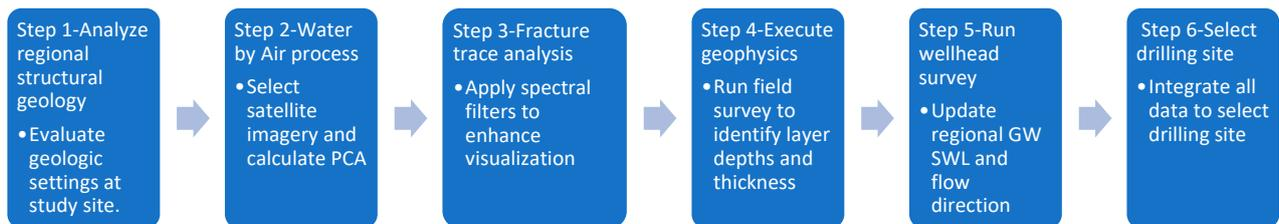
**Figure 7.** Workflow for a multi-technique framework for groundwater prospecting.
