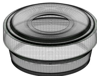
Figure 4. Updated mesh of the 0.5 mm radial installation deviation model.
