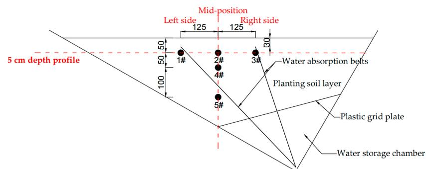
Figure 3. The water content measuring points in the slab trench model with water absorption belts (unit: mm).
