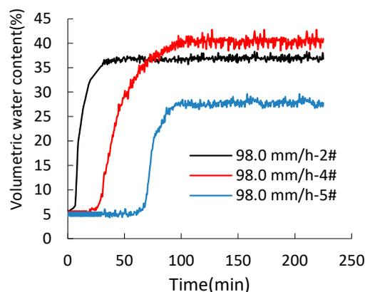
**Figure 11.** Response of volumetric water content along the depth of the middle axis in the models (2#, 4#, 5#) with one strain of plant under rainfall intensity of 98.0 mm/h.
