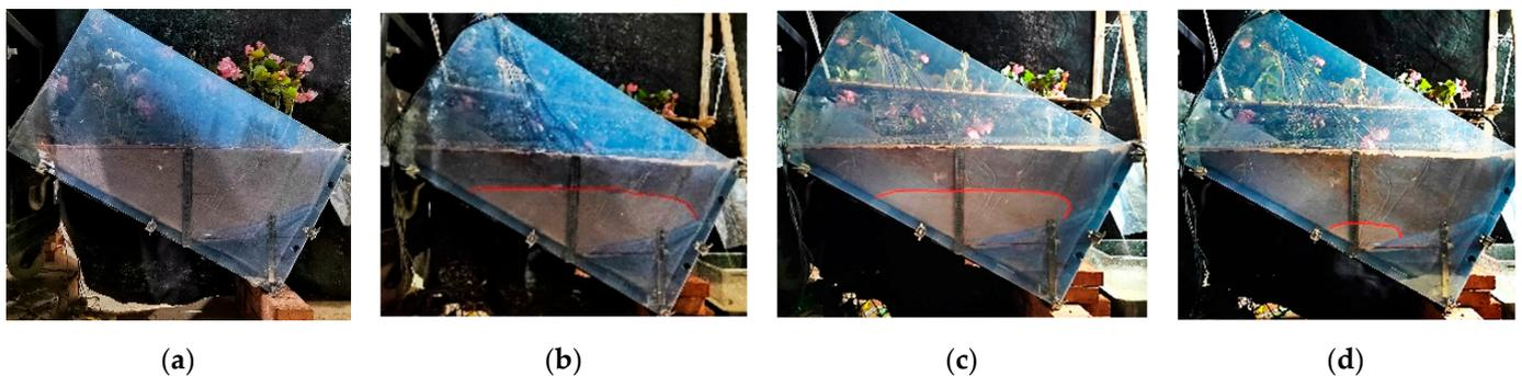
**Figure 6.** The wetting front observed at different moment in the model with rainfall intensity of 222 mm/h and 3 strains of plants: (a) 0 min; (b) 30.0 min; (c) 50.0 min; (d) 90.0 min.
