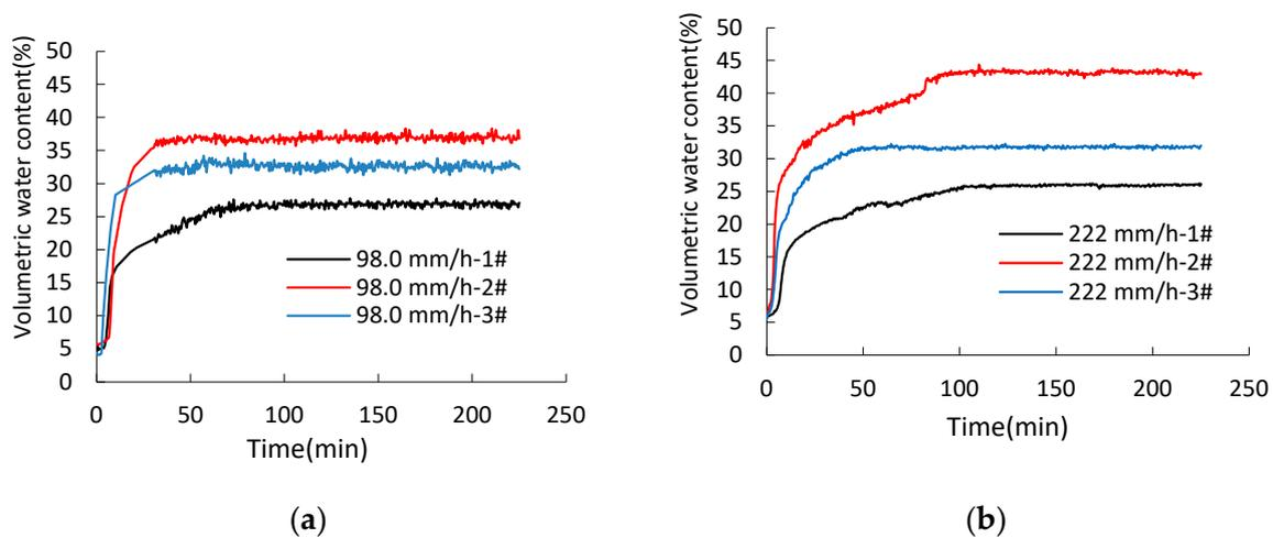
**Figure 12.** Response of volumetric water content at 5 cm sub-surface along the width direction in the models (1#, 2#, 3#) with one strain of plant under different rainfall intensity: (a) Relationship curve of volumetric water content versus time under rainfall intensity of 98.0 mm/h; (b) Relationship curve of volumetric water content versus time under rainfall intensity of 222 mm/h.
