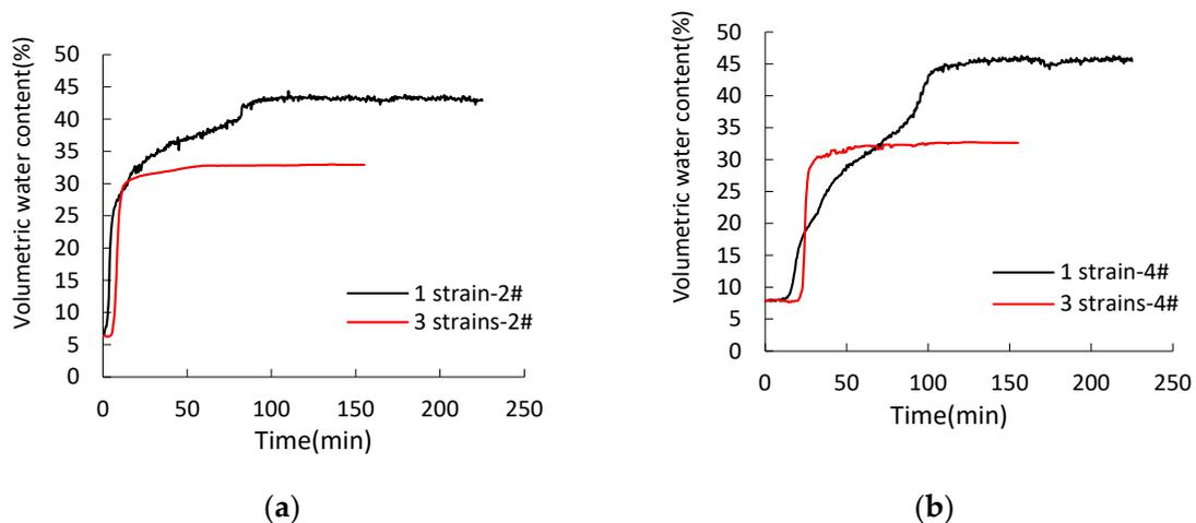
**Figure 10.** Response of volumetric water content along the depth of the middle axis in the model with different strains of plants under rainfall intensity of 222 mm/h: (a) Relationship curve of volumetric water content versus time measured by sensor 2# near the dense root area; (b) Relationship curve of volumetric water content versus time measured by sensor 4# near the root tip area.
