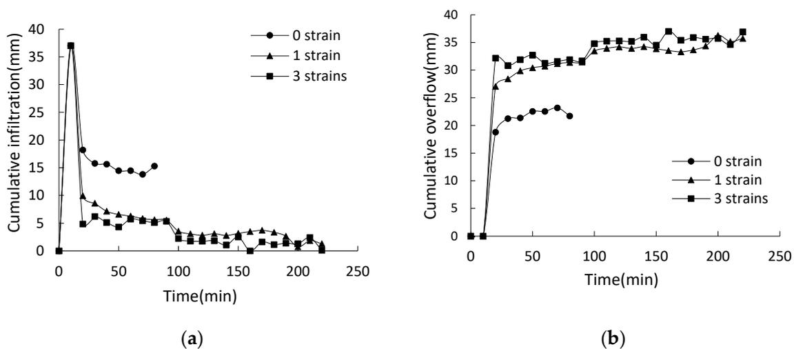
**Figure 8.** Time-history curves of rainfall infiltration and overflow amount under rainfall intensity of 222 mm/h in the models with different numbers of plants: (a) Relationship curve of cumulative infiltration amount versus time; (b) Relationship curve of cumulative water overflow versus time.
