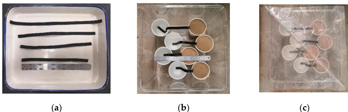
**Figure 5.** Water absorption model test of the absorption belts: (a) Water absorption belts used in the test; (b) Cups full of dry soil or water connected by absorption belts with different initial lengths exposed to air; (c) Model test on water absorption through belts.
