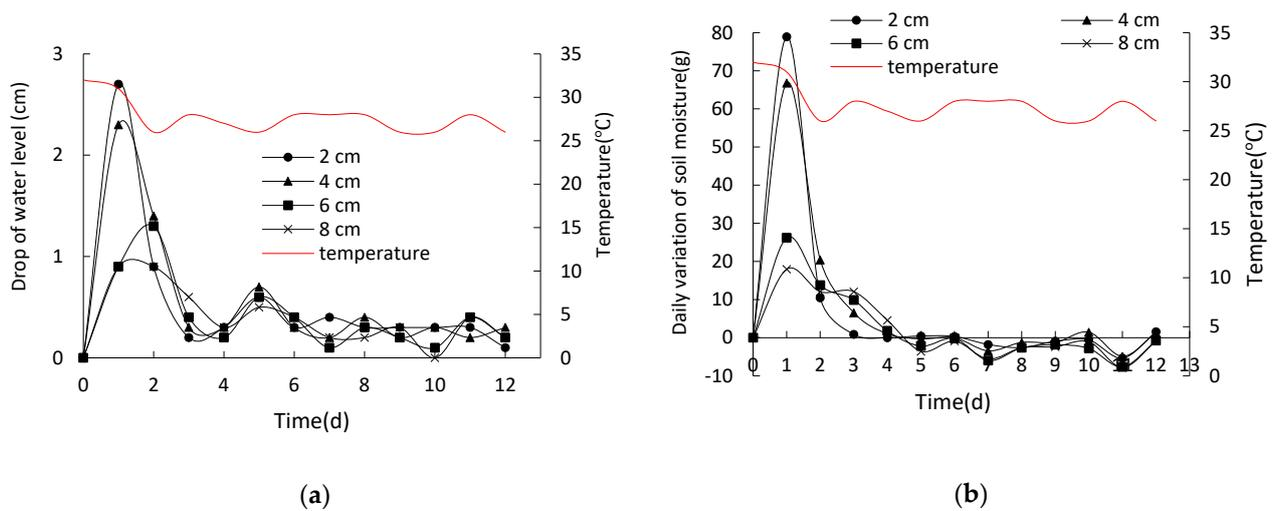
**Figure 18.** Results of water absorption test with different initial air-exposed lengths of absorption belts: (a) Relationship curve of water level drop in the cup and temperature change versus time; (b) Relationship curve of daily variation in soil moisture and temperature change versus time.
