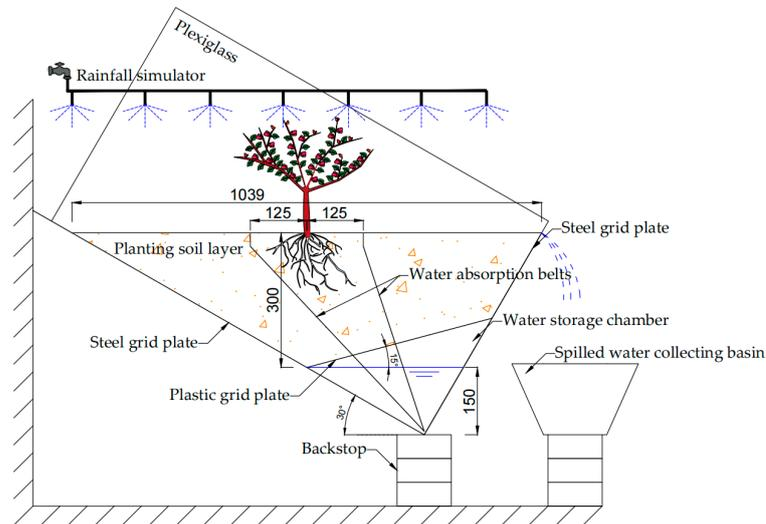
Figure 2. Model design diagram of the slab trench (unit: mm).
