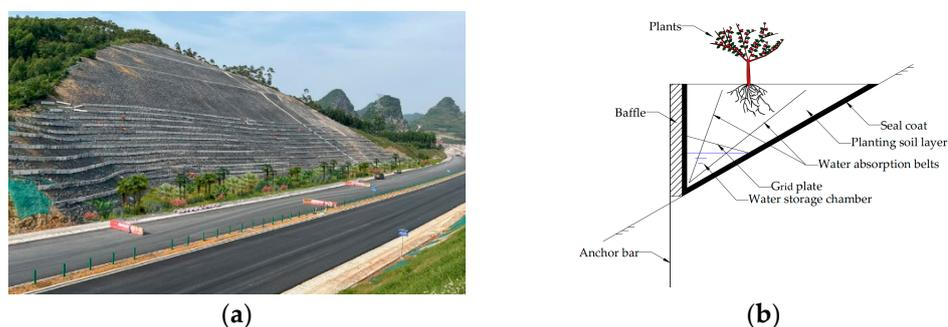
**Figure 1.** Slab trench arrangement and detailed structure: (a) In situ construction of stepped slab trench on the rocky desertification slope; (b) Profile of the slab trench.
