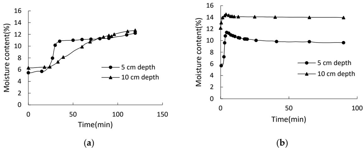
**Figure 19.** Response of moisture content at 5 cm and 10 cm sub-surface with time in rainfall stage with water stored in different plants: (a) Relationship curve of moisture content versus time in group 1 with water stored in succulent root plant; (b) Relationship curve of moisture content versus time in group 2 with water stored in succulent STEM plant.
