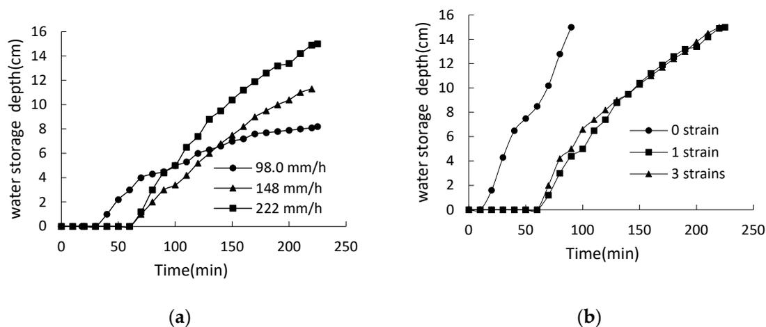
**Figure 9.** Variation curves of water storage depth versus time in the models with different rainfall intensity or different strains of plants in rainfall stage: (a) Relationship curve of water storage depth versus time with 1 strain of plant; (b) Relationship curve of water storage depth versus time under rainfall intensity of 222 mm/h.
