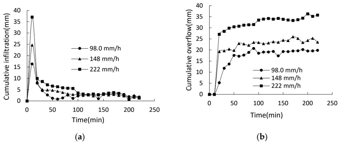
**Figure 7.** Time-history curves of rainfall infiltration and overflow amount under different rainfall intensities in the model: (a) Relationship curve of cumulative infiltration amount versus time; (b) Relationship curve of cumulative water overflow versus time.
