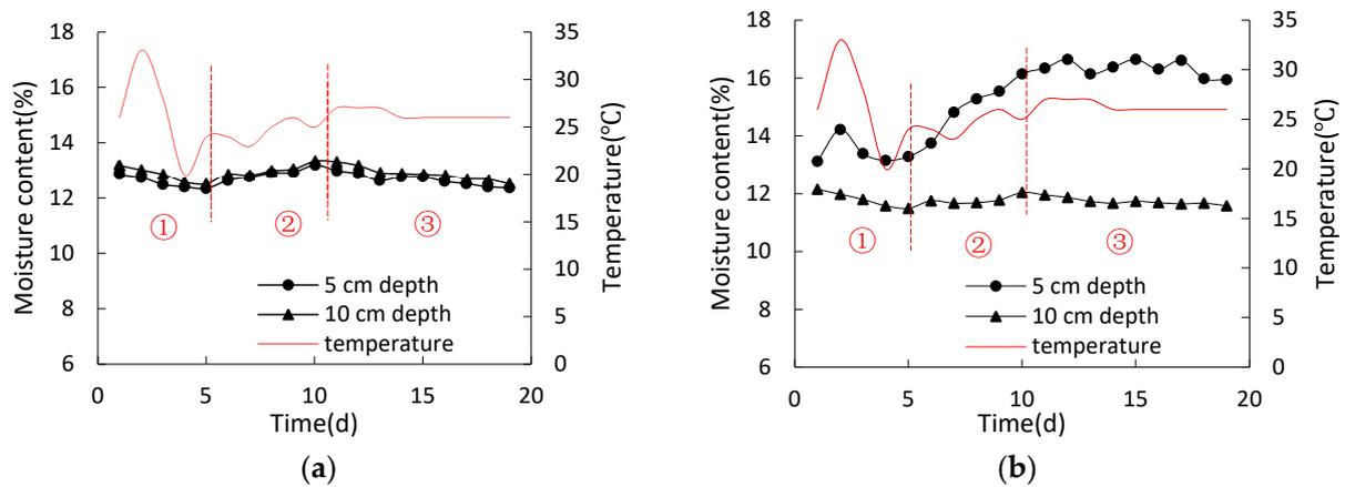
**Figure 20.** Response of moisture content at 5 cm and 10 cm sub-surface with time and temperature in drying stage with water stored in different plants: (a) Relationship curve of moisture content and temperature versus time in group 1 with water stored in succulent root plant; (b) Relationship curve of moisture content versus time in group 2 with water stored in succulent STEM plant.
