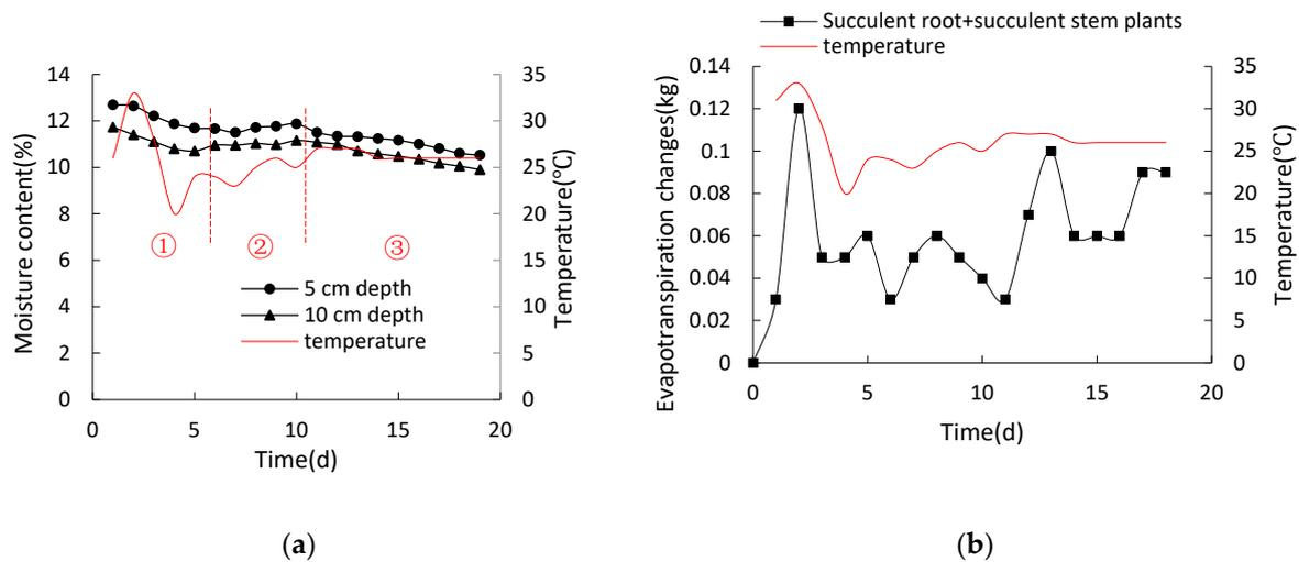
**Figure 22.** Response of water change with time and temperature in group 3 with water stored in both succulent root and succulent stem plants in drying stage: (a) Relationship curve of moisture content and temperature versus time at 5 cm and 10 cm sub-surface; (b) Relationship curve of evapotranspiration change and temperature versus time.
