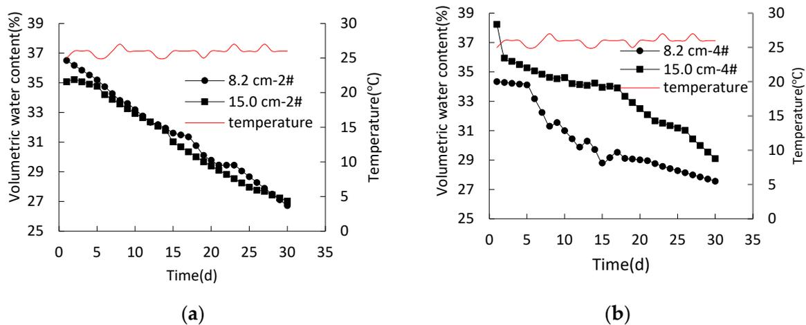
**Figure 16.** Response of volumetric water content along the depth of the middle axis in test groups MT1 and MT3 with one strain of plant during drying period after rainfall, which formed different initial water storage depths of 8.2 cm or 15.0 cm: (a) Relationship curve of volumetric water content versus time measured by sensor 2# near the dense root area; (b) Relationship curve of volumetric water content versus time measured by sensor 4# near the root tip area.
