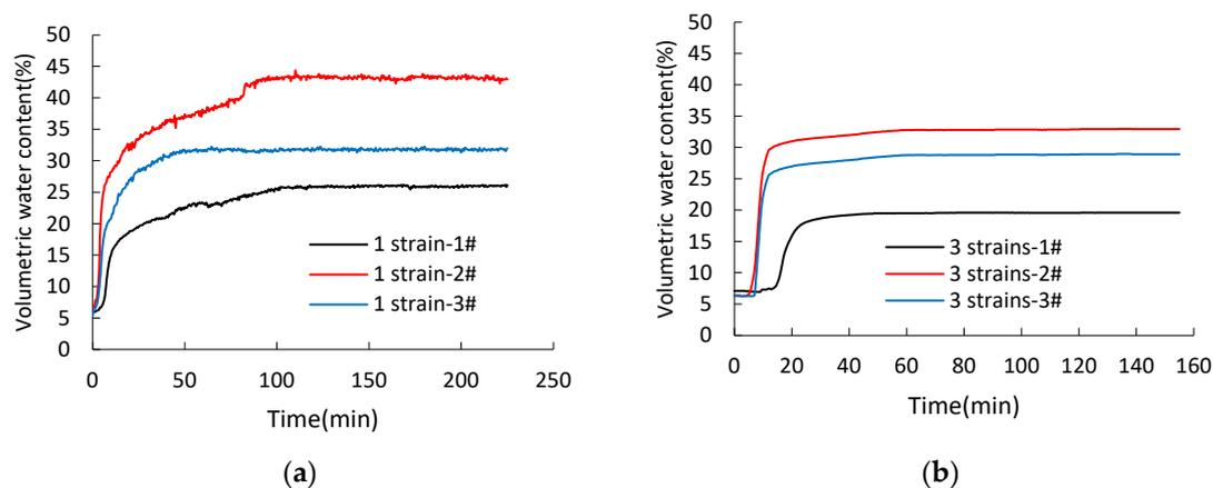
**Figure 13.** Response of volumetric water content at 5 cm sub-surface along the width direction in the models (1#, 2#, 3#) with different strains of plants under rainfall intensity of 222 mm/h: (a) Relationship curve of volumetric water content versus time with one strain of plant; (b) Relationship curve of volumetric water content versus time with three strains of plant.
