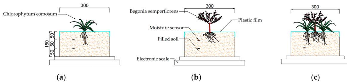
**Figure 4.** Side view of the models with different kinds of plants in drought state: (a) Succulent root plant; (b) Succulent stem plant; (c) Succulent root and stem plant in a mixed manner (unit: mm).
