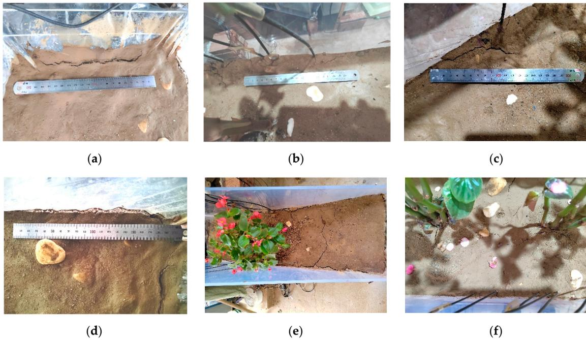
**Figure 14.** Crack development on the surface of soil: (a) Surface crack due to wetting collapse after rainfall; (b) Drying tiny cracks at the edge; (c) tiny cracks after further drying; (d) Shrinkage cracks at the edge; (e) Cracks in the middle; (f) Tiny cracks between plants.
