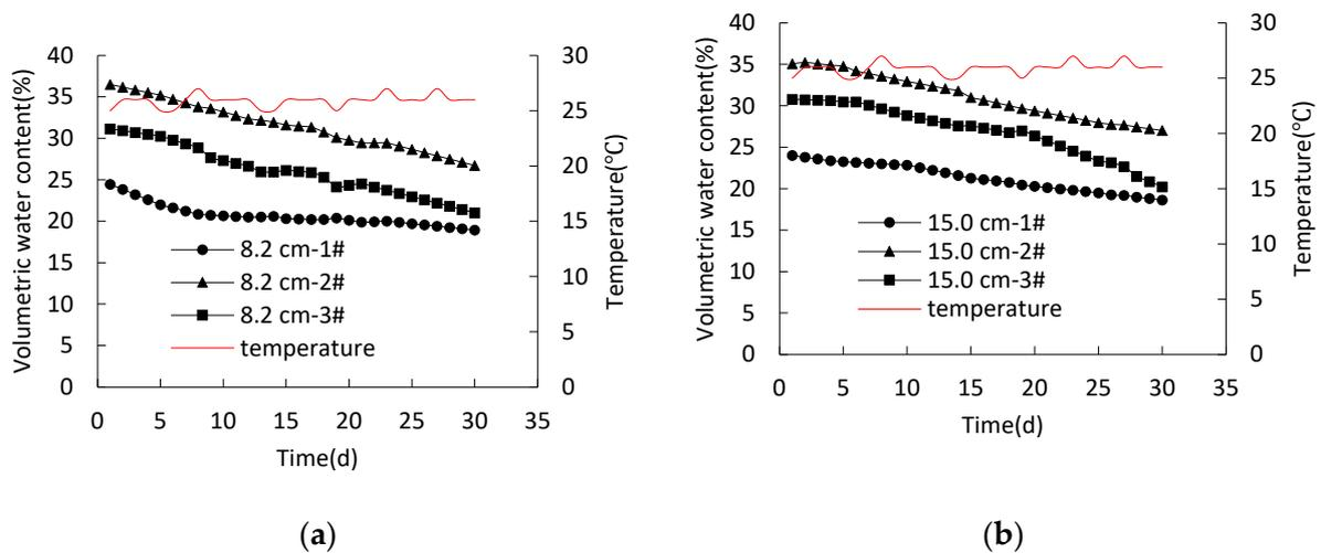
**Figure 17.** Response of volumetric water content at 5 cm sub-surface along the width direction in the models (1#, 2#, 3#) with one strain of plant during drying period after rainfall, which formed different initial water storage depths: (a) Relationship curve of volumetric water content versus time with initial water storage depth of 8.2 cm; (b) Relationship curve of volumetric water content versus time with initial water storage depth of 15.0cm.
