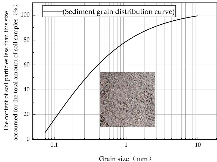
**Figure 1.** Deposit sediment photo and particle gradation curve.
