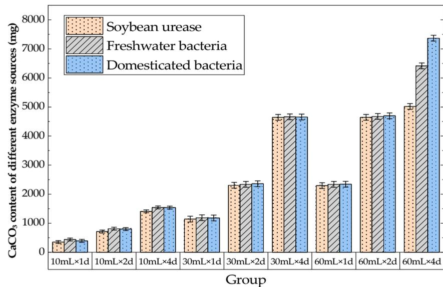
**Figure 5.** Calcium carbonate production 72 h after seawater injection.
