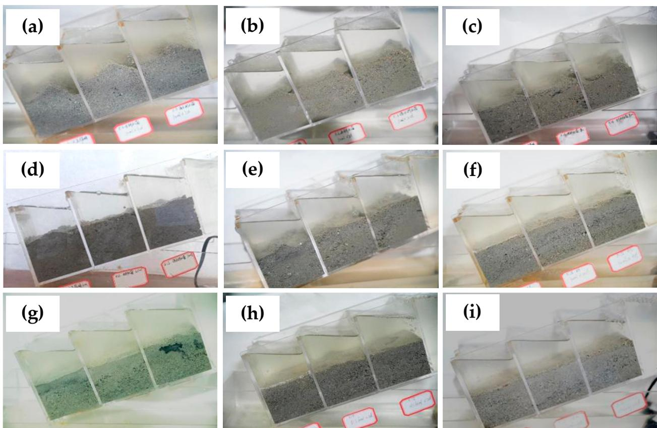
**Figure 8.** A 4 h wash-out plot after curing of different enzyme sources. (Corresponding sample number in Table 2: (a) 1–10; (b) 2–10; (c) 4–10; (d) 1–30; (e) 2–30; (f) 4–30; (g) 1–60; (h) 2–60; (i) 4–60).
