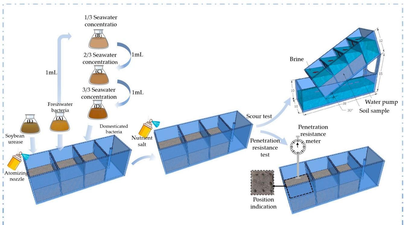
**Figure 2.** Scour and penetration resistance test.
