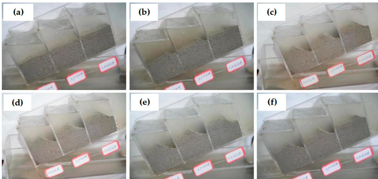
**Figure 7.** Change in untreated coastal sand scouring (Scour time: (a) 0 min; (b) 1 min; (c) 30 min; (d) 1 h; (e) 2 h; (f) 4 h).
