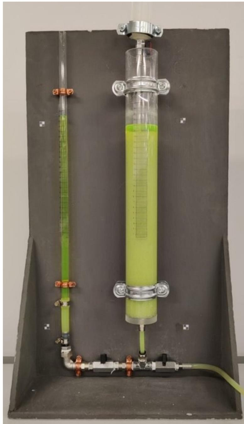
**Figure 1.** Experimental equipment for the column filled with glass beads of 1 mm diameter as the porous media and saturated with water and fluorescein.
