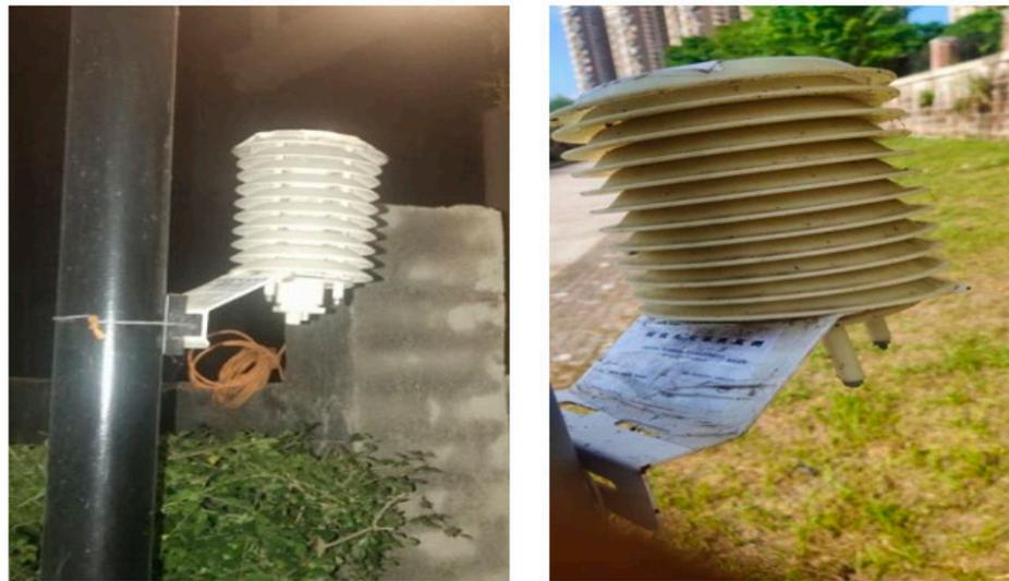
**Figure 3.** Small HOBO weather station.
