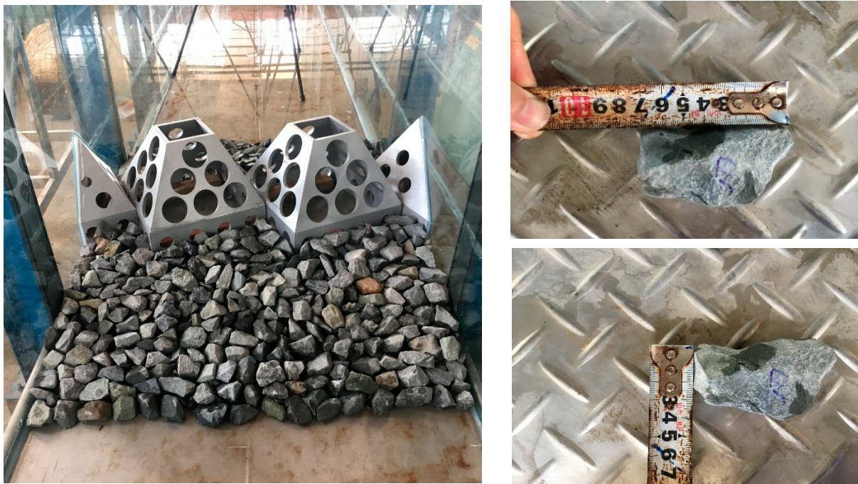
Figure 9. Design of stone revetment for scour protection.
