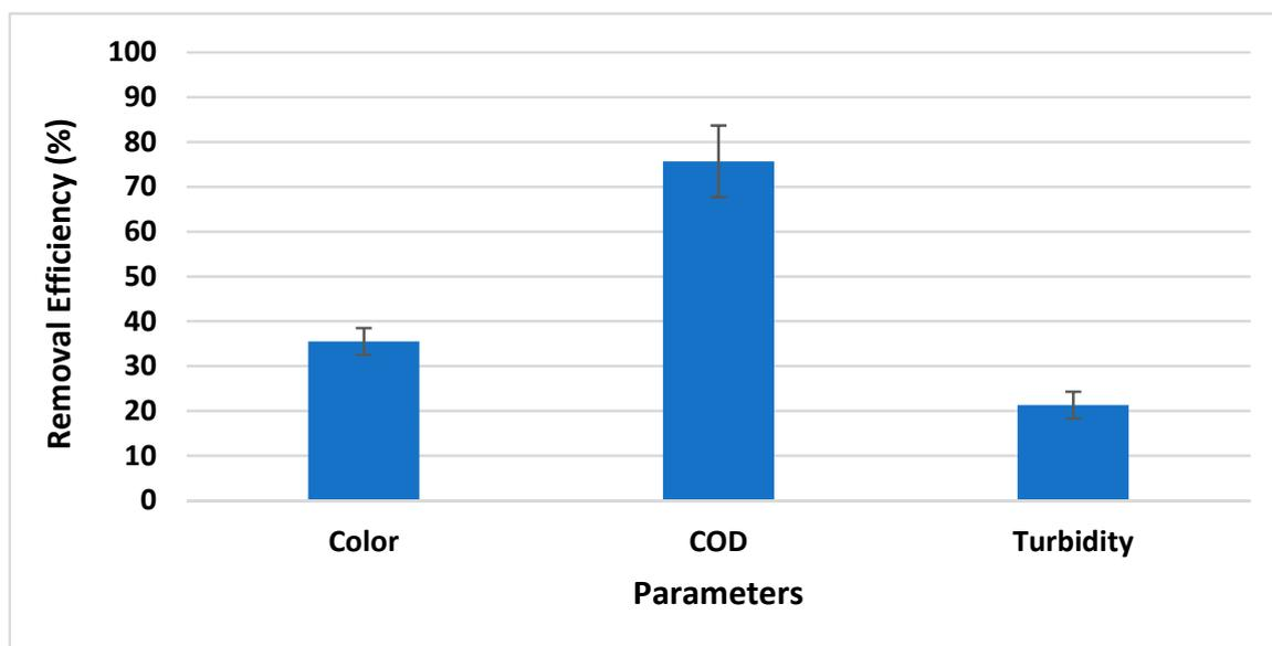
**Figure 8.** Fenton oxidation of chemically treated wastewater for removal of color, COD and turbidity. Means values are presented with standard deviation.
