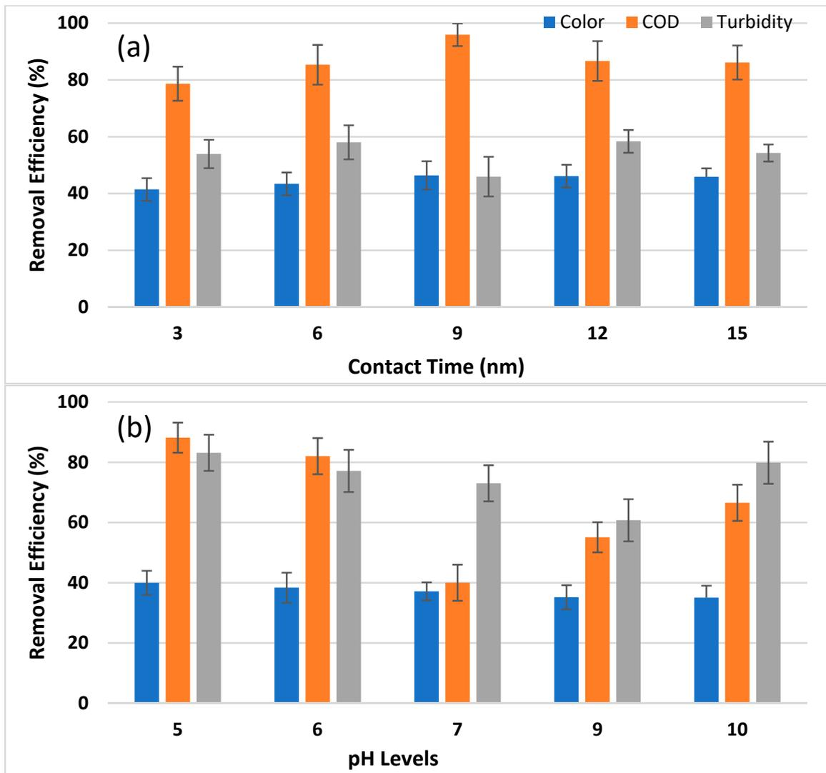
**Figure 4.** (a) Ozone treatment of biologically treated wastewater and removal efficiencies (%) for color, COD and turbidity at varying contact times of 3, 6, 9, 12 and 15 min. (b) Ozone treatment of biologically treated wastewater and removal efficiencies (%) for color, COD and turbidity at varying pH values (5, 6, 7, 9 and 10). Means values are presented in graphs with standard deviation.
