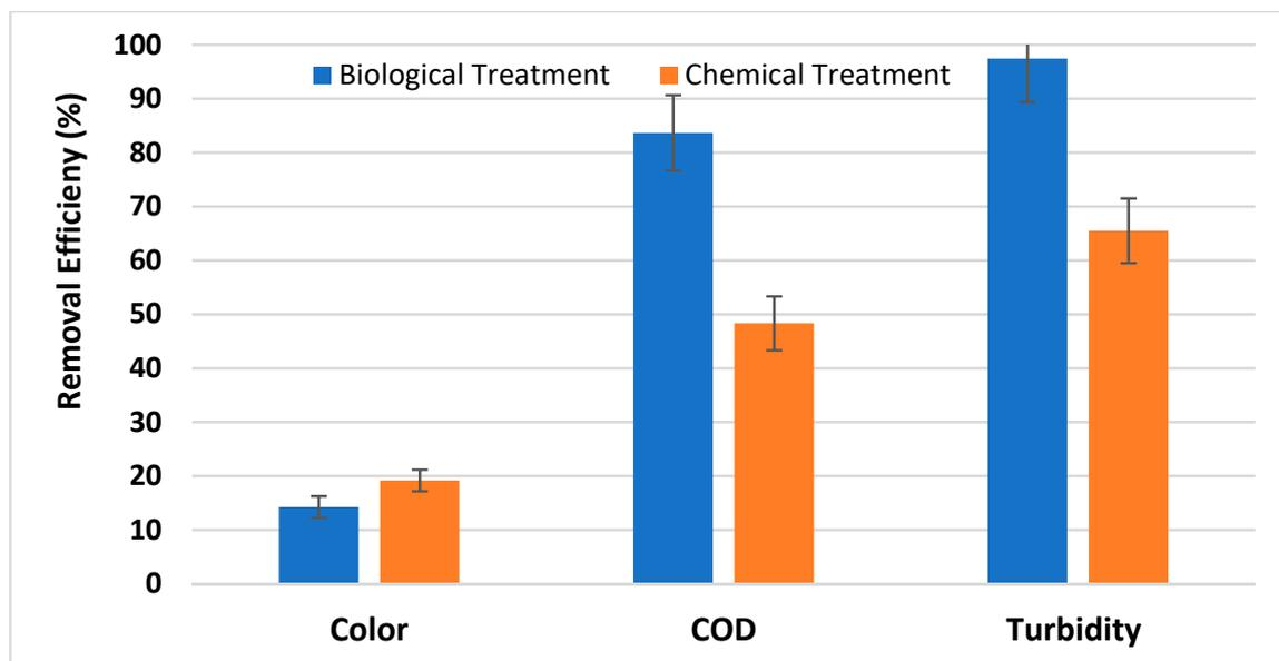
**Figure 2.** Removal efficiencies of biological treatment and chemical treatment of wastewater from pulp and paper industry for color, COD and turbidity. Mean values of percent removal of pollutant are presented with standard deviation.
