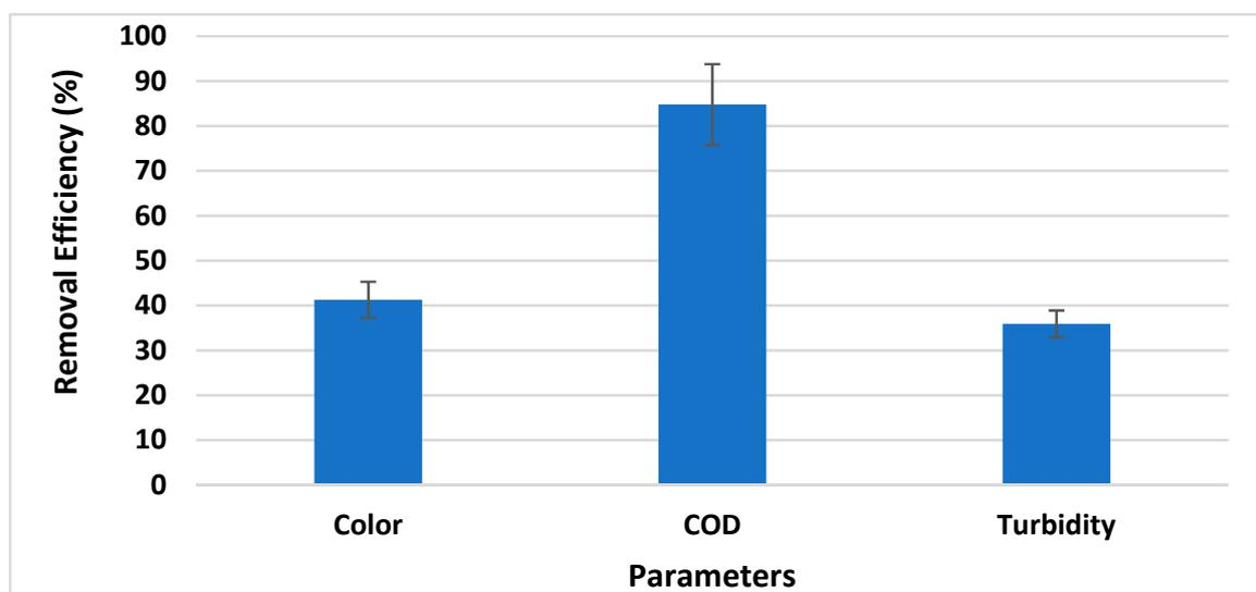
**Figure 5.** Ozone treatment of chemically treated wastewater and removal efficiencies (%) for color, COD and turbidity. Means values are presented in graphs with standard deviation.
