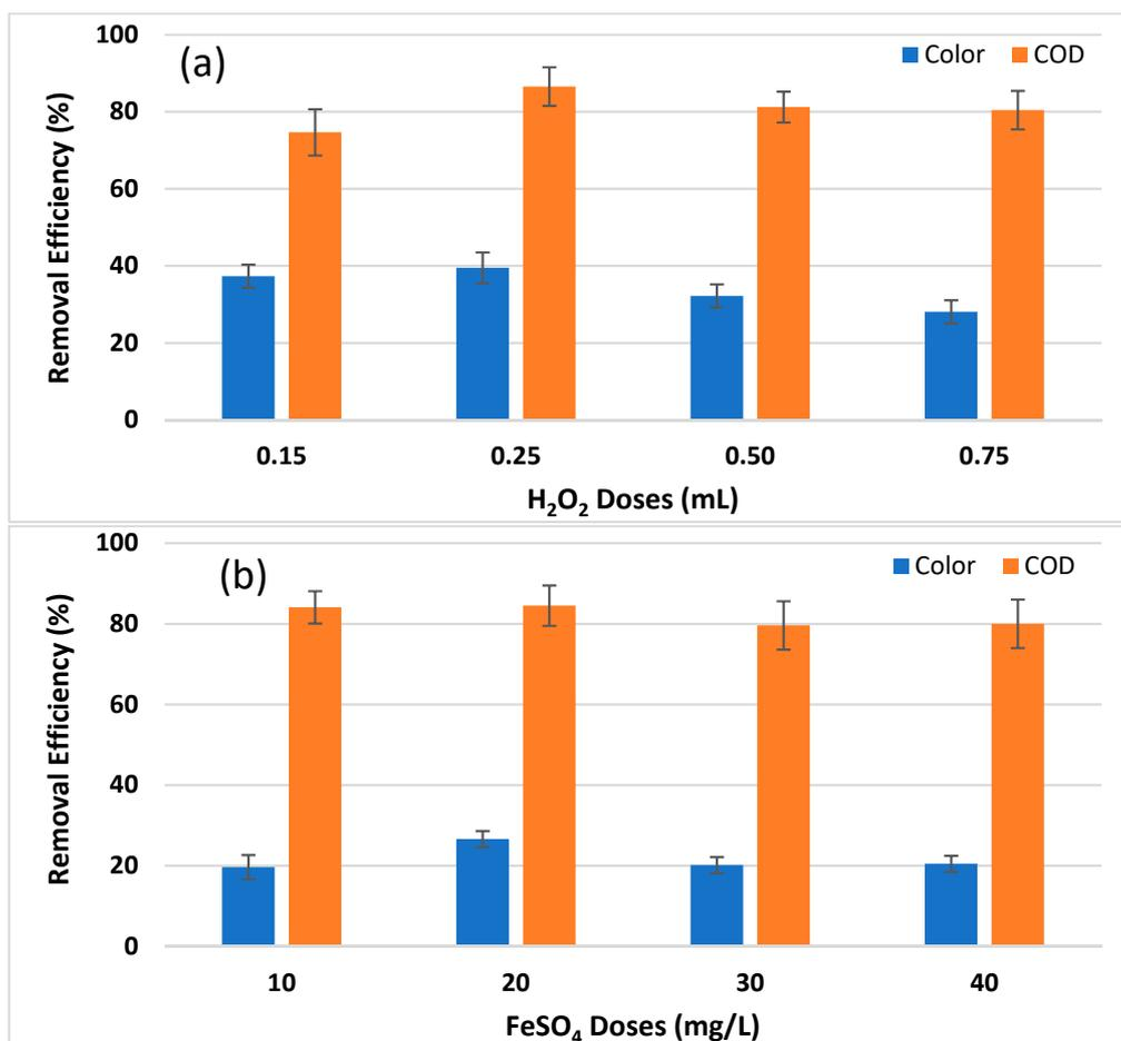
**Figure 7.** (a) Optimization of H<sub>2</sub>O<sub>2</sub> dose of treated pulp and paper wastewater for Fenton oxidation at different doses (0.15, 0.25, 0.50 and 0.75 mL) for biologically treated wastewater. (b) Optimization of FeSO<sub>4</sub> dose of treated pulp and paper wastewater for Fenton oxidation at different doses (10, 20, 30 and 40 mg/L) for biologically treated wastewater. Means values are presented with standard deviation.
