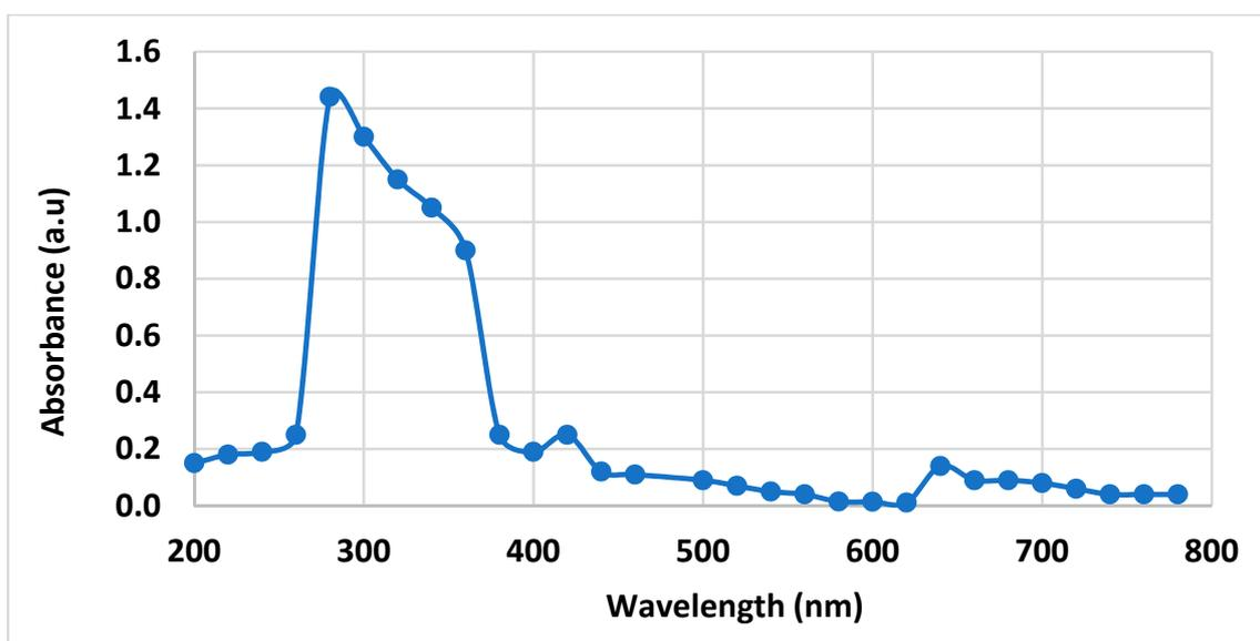
**Figure 1.** Absorption spectrum of raw wastewater from paper industry in the UV/Vis range.
