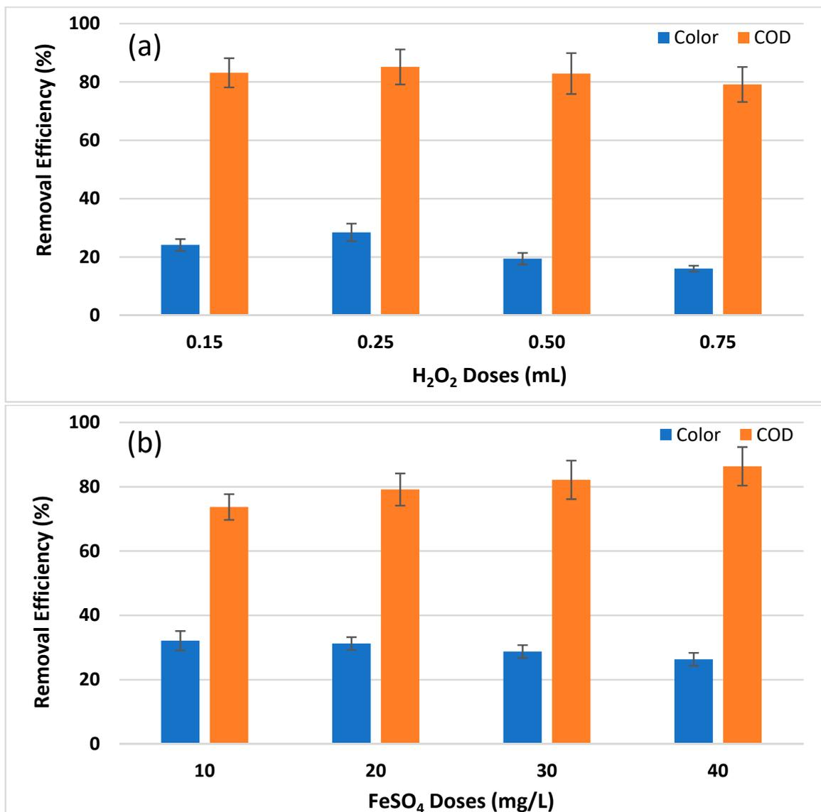
**Figure 6.** (a) Optimization of H<sub>2</sub>O<sub>2</sub> dose of raw pulp and paper wastewater for Fenton oxidation at different doses (0.15, 0.25, 0.50 and 0.75 mL). (b) Optimization of FeSO<sub>4</sub> dose of raw pulp and paper wastewater for Fenton oxidation at different doses (10, 20, 30 and 40 mg/L). Means values are presented with standard deviation.
