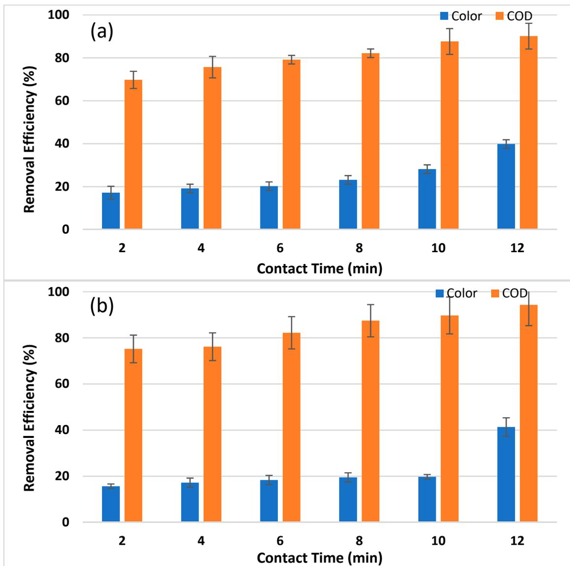
**Figure 9.** (a) Photo-Fenton treatment of raw pulp and paper wastewater and its removal efficiency for color and COD at different contact times of 2, 4, 6, 8, 10 and 12 min. (b) Photo-Fenton treatment of biologically treated pulp and paper wastewater and its removal efficiency for color and COD at different contact times of 2, 4, 6, 8, 10 and 12 min. Means values are presented with standard deviation.
