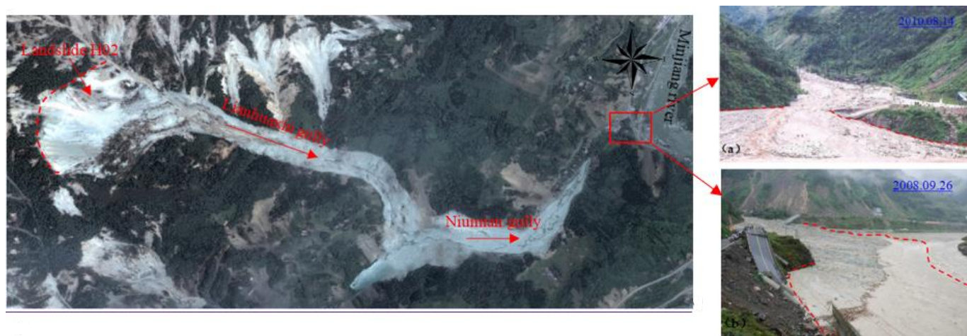
Figure 4. Characteristics of debris flow fans at the gully mouth: (a) “8.14” debris flow fan; and (b) “9.26” debris flow fan. (The arrows on the left show the direction of the slide, and the arrows on the right show an enlarged view of two debris flows in the area).
