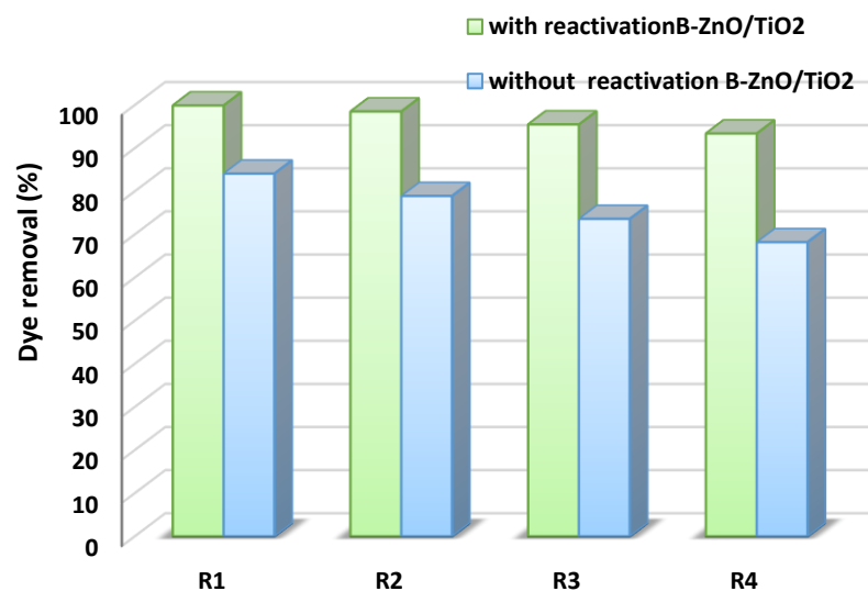
Figure 15. Cycling runs of B-ZnO/TiO 2 for the photodegradation of DR16 with and without reactivation.
