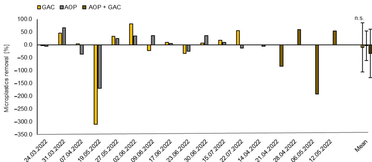
**Figure 2.** Measured microplastics' removal using GAC and AOP in parallel and series connection (AOP before GAC). The reduction is measured as the difference in microplastics' concentrations between the influent and effluent of the fourth cleaning step. Every sample was performed as a duplicate. n.s.—not statistically significant, *t*-test, paired, 1-sided,  $p < 0.05$ .
