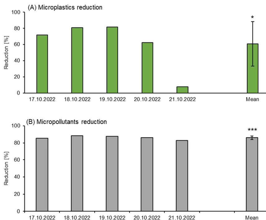
**Figure 3.** Removal of (A) microplastics and (B) micropollutants within the pilot plant trails for organosilane-induced microplastics removal combined with GAC. The reduction is measured as the difference in concentrations between the influent and effluent of the fourth cleaning step. \* =  $p < 0.05$ ; \*\*\* =  $p < 0.001$ ,  $t$  test, paired, 1-sided.
